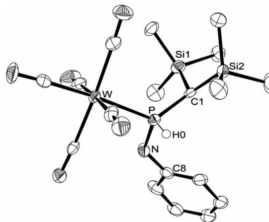
Figure 3. Molecular structure of complex **3e** in the crystal. All hydrogen atoms except Hp are omitted for clarity. Selected bond lengths [Å] and bond angles [°]: P–N 1.691(11), P–C1 1.835(13), P–W 2.516(3), N–C8 1.430(18); N–P–C1 107.8(6), C1–P–W 127.1(4), W–P–N 108.0(4).
