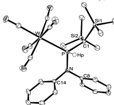
Figure 1. Molecular structure of complex **3c** in the crystal. All hydrogen atoms except Hp are omitted for clarity. Selected bond lengths [Å] and bond angles [°]: P–Hp 1.29(3), P–W 2.5305(7), P–N 1.717(2), P–C1 1.819(3), N–C8 1.488(3); N–P–W 118.13(8), N–P–C1 104.09(11), W–P–C1 121.58(9).
