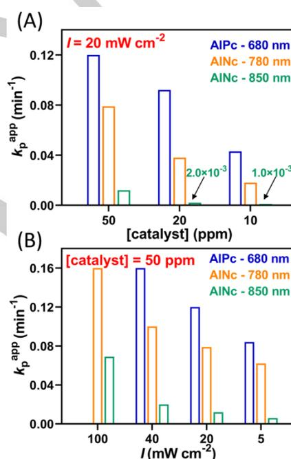
**Figure 2.** (A) Evolution of apparent propagation rates ( $k_p^{\text{app}}$ ) of MA polymerizations with increasing AIPc and AINc concentrations under 680, 780 and 850 nm light at a fixed intensity of  $20 \text{ mW cm}^{-2}$ . (B) Evolution of  $k_p^{\text{app}}$ 's of MA photopolymerizations with increasing light intensity ( $5\text{-}100 \text{ mW cm}^{-2}$ ) using fixed AIPc and AINc concentrations under 680, 780 and 850 nm light.
