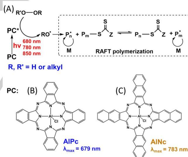
**Scheme 1.** (A) Long wavelength photosensitization of (hydro)peroxides to generate radicals under far-red and NIR wavelengths mediated by (B) aluminum phthalocyanine (AIPc) and (C) aluminum naphthalocyanine (AINc).
