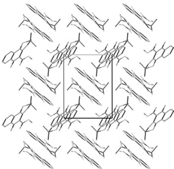
**Fig. 3.** Packing scheme for mollugin. Projection along  $c$ -axis.
