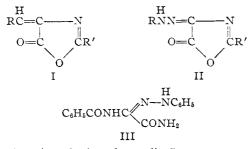
4-Phenylazo-2-phenyloxazolin-5-one, according to Kuskov,<sup>2</sup> decomposes in boiling alcoholic ammonia to give III. Kuskov's nitrogen analysis, 21.4%, does not agree with the calculated value for the composition just given, and in these Laboratories it was found that the expected hydrazone band, 360–370 m $\mu$ , is missing in the reaction product.
