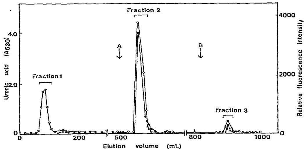
Fig. 3. Separation of fluorescent heparin into 5-aminofluorescein-labeled and unlabeled fractions on Octyl-Sepharose CL-4B. Fluorescent heparin (degree of substitution 0.039) (100 mg) was chromatographed according to the same procedure as described in the legend to Fig. 2, except for the stepwise elution system of 3.0M (3.5 bed vol.), M (A, 2.5 bed vol.), and no ammonium sulfate in 50mM phosphate buffer (B, 1.4 bed vol.).
