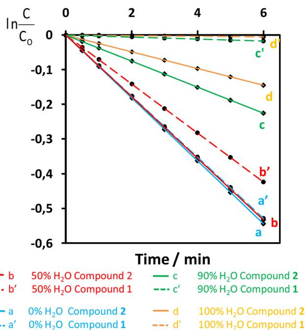
**Fig. 4.** Comparison of pseudo-first order linear fitting for the production of  $^1\text{O}_2$  by **1** and **2** in different media (CH<sub>3</sub>CN/H<sub>2</sub>O).
