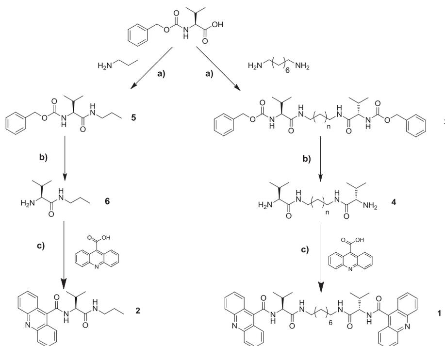
Scheme 1. Synthetic route for compounds **1** and **2** a) THF,  $\text{Et}_3\text{N}$  ClCOOEt, r.t., 12 h b)  $\text{CH}_3\text{OH}$ , Pd/C  $\text{H}_2$ , r.t., 6 h c) for acridine-9-carboxylic acid activation:  $\text{CH}_2\text{Cl}_2$ , oxalyl chloride, DMF(cat). For activated acid and amine coupling reaction: THF,  $\text{Et}_3\text{N}$ , 16 h.
