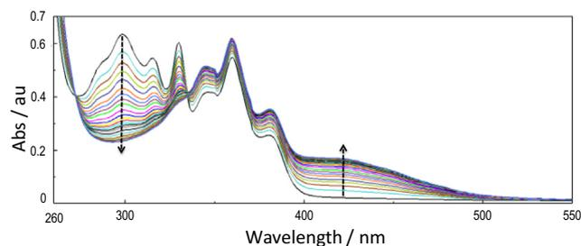
**Fig. 3.** Photooxidation of DHN by  $^1\text{O}_2$  induced by irradiation of **1** in CH<sub>3</sub>CN, monitored by UV-Vis spectroscopy. [DHN] = 80  $\mu\text{M}$ ; [**1**] = 33  $\mu\text{M}$ .
