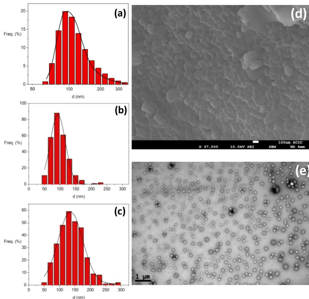
**Fig. 6.** (a) Representative DLS analysis of **1** aggregates; (b) SEM analysis of **1** aggregates; (c) TEM analysis of **1** aggregates; (d) SEM micrograph of **1**; (e) TEM micrograph of **1**.
