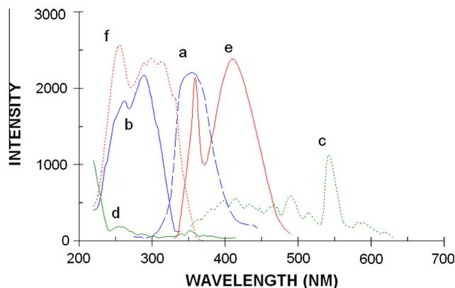
Fig. 4. a > Ce<sup>3+</sup> Emission for 290 nm excitation. b > Excitation for 358 nm emission of LiBaF<sub>3</sub>:Ce<sup>3+</sup> c > Tb<sup>3+</sup> Emission for 220 nm excitation. d > Excitation for 543 nm emission of LiBaF<sub>3</sub>:Tb<sup>3+</sup> e > Eu<sup>2+</sup> Emission for 320 nm excitation. f > Excitation for 410 nm emission of LiBaF<sub>3</sub>:Eu<sup>2+</sup>.
