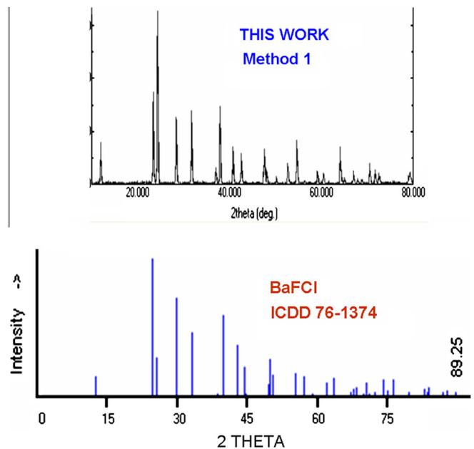
Fig. 1. XRD pattern of attempted LiBaF<sub>3</sub> using method 1 (precipitation from aqueous chloride solution using HF) When precipitation synthesis of LiBaF<sub>3</sub> was attempted from aqueous solutions of LiCl and BaCl<sub>2</sub>, using HF as precipitating agent, BaFCl is formed as shown by excellent matching with ICDD data file 76-1374.
