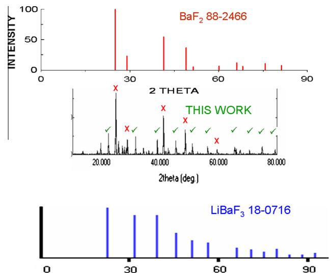
Fig. 2. XRD pattern of attempted LiBaF<sub>3</sub> using method 2 (precipitation from aqueous acetate solution using HF). When precipitation synthesis of LiBaF<sub>3</sub> was attempted from aqueous solutions of lithium and Barium acetates, using HF as precipitating agent, mixed phase compound was formed. The phases can be identified as BaF<sub>2</sub> (marked by crosses, ICDD data file 88-2466), and LiBaF<sub>3</sub> (marked by tick marks, ICDD data file 18-0176).
