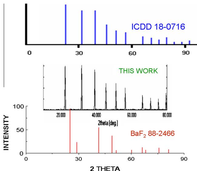
Fig. 3. XRD pattern of LiBaF<sub>3</sub> using method 3. An excellent match with ICDD data file 18-0716 is seen.
