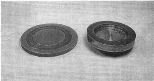
Fig. 3—Example PS304-coated steel disk (left) and washer surface of Inconel X-750 ring following thrust-washer testing, with circular track worn into PS304 coating.
