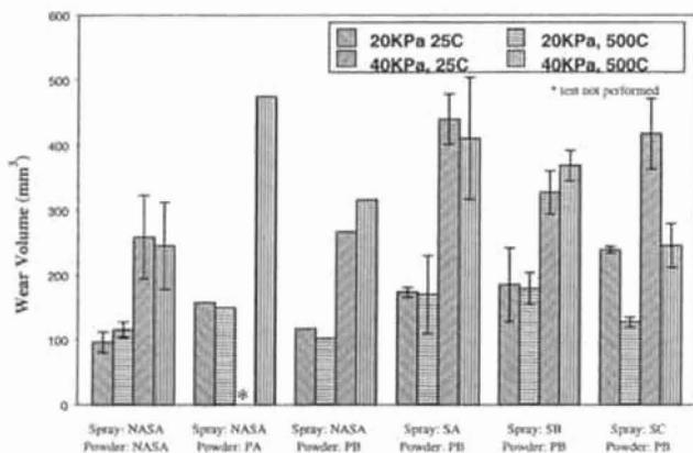
Fig. 6—Wear volumes from PS304 coatings deposited at various spray facilities (NASA, SA, SB and SC) using various powder mixtures (NASA-prepared and RPI-prepared PA or PB) sliding against Inconel X-750 during thrust-washer tests at various combinations of contact pressure (20 or 40kPa) and temperature (ambient or 500°C).
