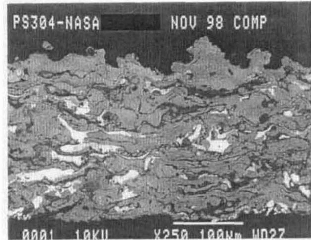
Fig. 5—Backscattered electron image of an example PS304 coating atop substrate at bottom, and unground surface at top.
