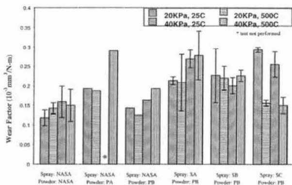
Fig. 7—Wear factors ( $\text{mm}^3/\text{Nm}$ ) of PS304 coatings deposited at various spray facilities (NASA, SA, SB and SC) using various powder mixtures (NASA-prepared and RPI-prepared PA or PB) sliding against Inconel X-750 during thrust-washer tests at various combinations of contact pressure (20 or 40kPa) and temperature (ambient or 500°C).
