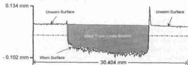
Fig. 4—Example stylus profile taken across PS304 wear track, illustrating wear track cross-sectional area.
