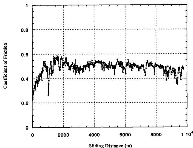
Fig. 2—Example friction coefficient record from a thrust-washer sliding test.
