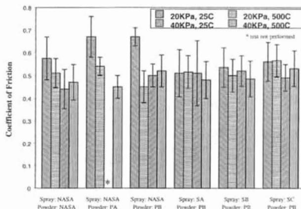
Fig. 8—Friction coefficients of PS304 coatings deposited at various spray facilities (NASA, SA, SB and SC) using various powder mixtures (NASA-prepared and RPI-prepared PA or PB) sliding against Inconel X-750 during thrust-washer tests at various combinations of contact pressure (20 or 40kPa) and temperature (ambient or 500°C).
