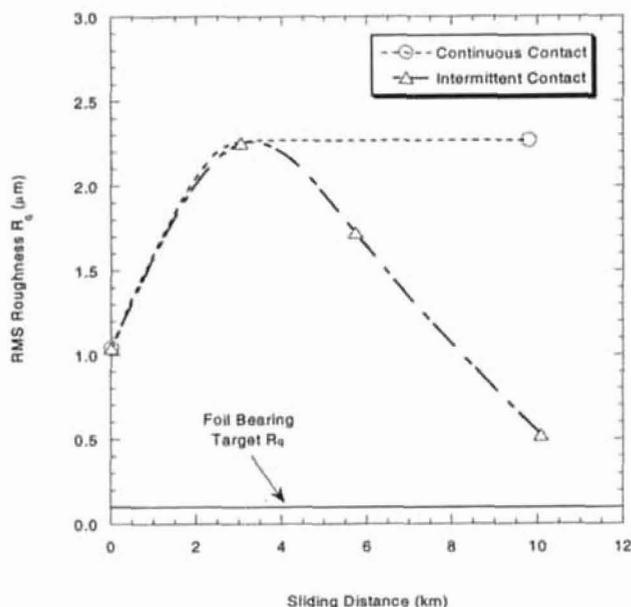
Fig. 11—Roughness of PS304 coating as a function of sliding distance during intermittent contact thrust-washer test at 500°C and 20kPa contact pressure. Also noted are roughness produced during typical continuous contact thrust-washer test at same temperature and pressure, as well as  $R_q=0.1\mu\text{m}$  target roughness of PS304 coatings for foil bearing applications, which is achieved during run-in under cyclic start/stop high-temperature operation.
