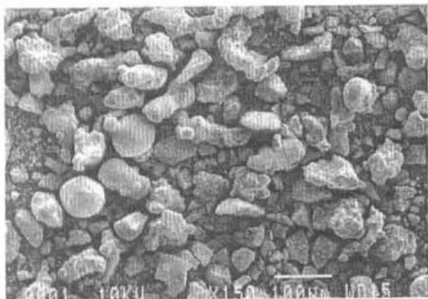
Fig. 1—Secondary electron image of an example PS304 powder mixture (PA).
