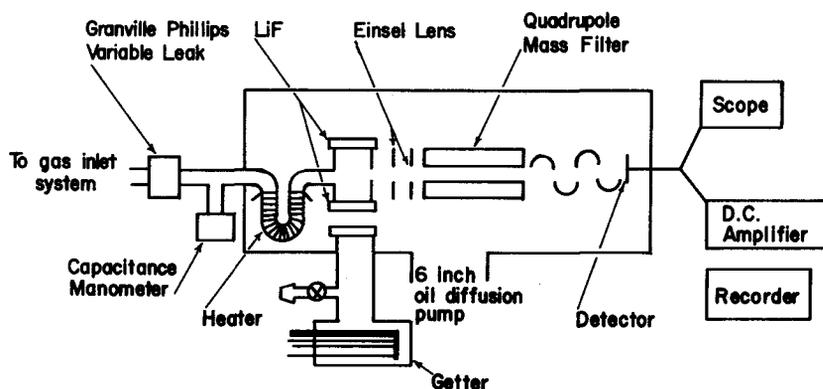
FIG. 1. Schematic drawing of the mass spectrometer.
