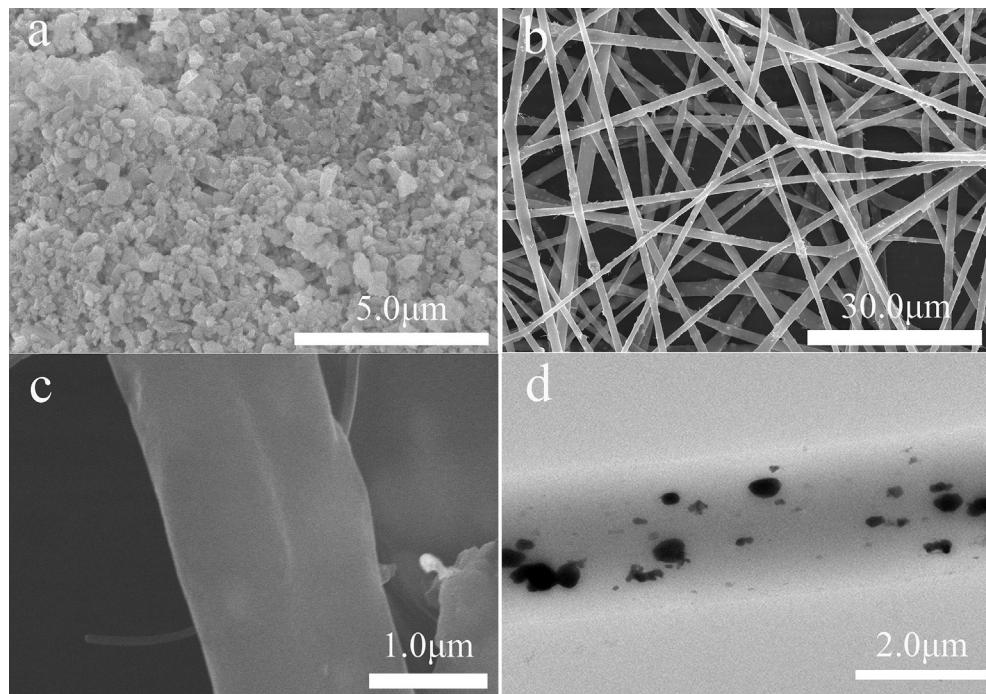
**Fig. 2.** SEM images of BSEN particles (a) and PVP/BSEN fibers (b, c) and TEM image of PVP/BSEN functional fiber (d).
