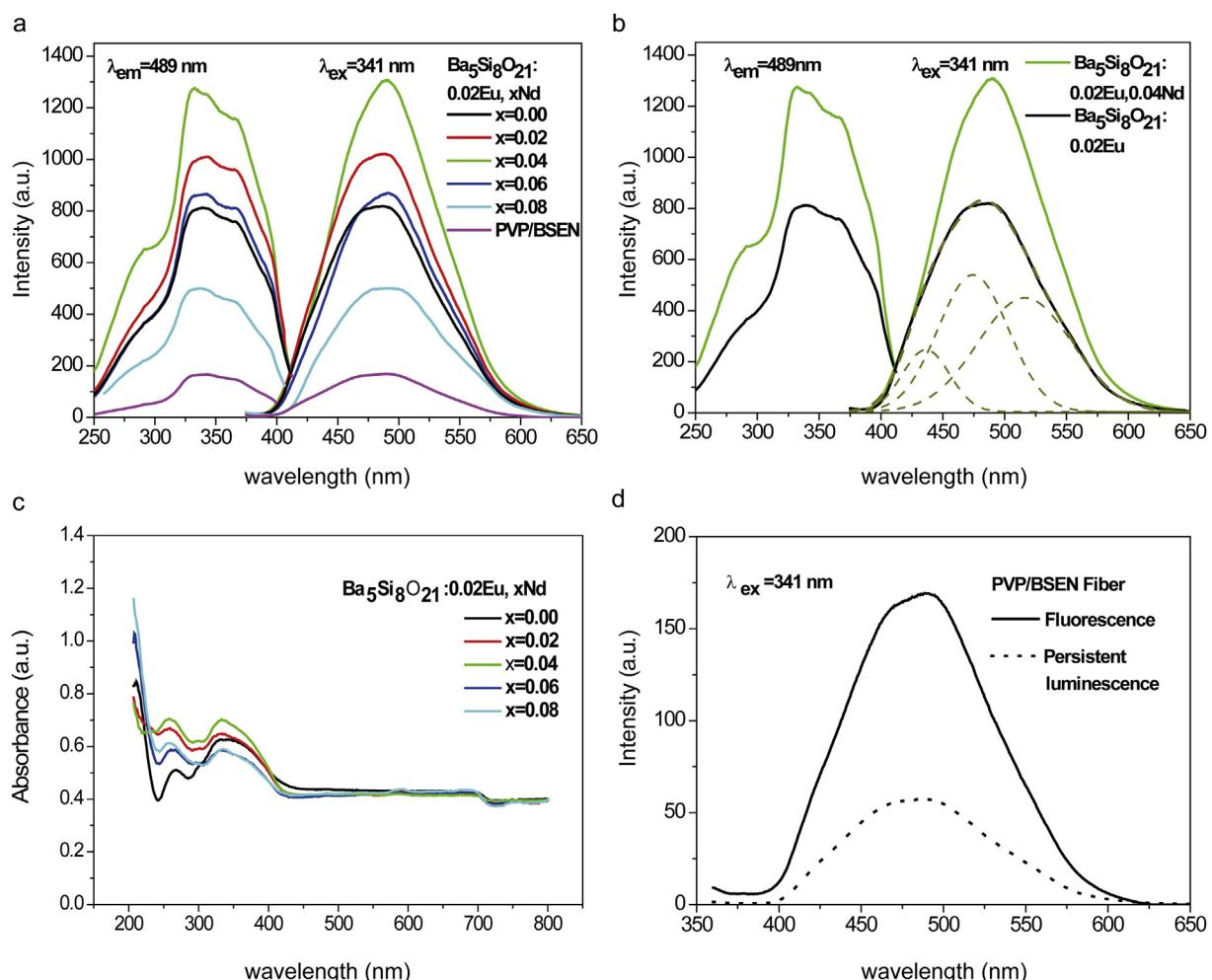
**Fig. 3.** Excitation and emission spectra of BSEN particles and PVP/BSEN fibers (a). Excitation and emission spectra of BSE and BSEN particles (b). Absorption spectra of BSEN particles (c). Fluorescence and persistent luminescence emission spectra (1 min after removing excitation) of PVP/BSEN fiber (d).
