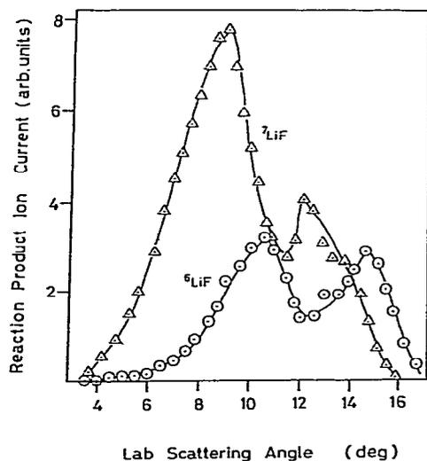
Fig. 6. Angular distribution of the isotopically selective reaction products LiF produced by the reaction with  $\text{CHClF}_2$ . The molecular isotopes detected  $^6\text{LiF}$  and  $^7\text{LiF}$ ; the atomic isotope excited is  $^6\text{Li}$ ; the state used is the excited  $2P_{3/2}$  state.
