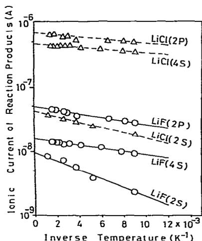
Fig. 4. Arrhenius plot for the reaction products LiF and LiCl with and without chemical reaction enhancement by laser irradiation. The molecular isotopes detected are LiF and LiCl; the atomic isotopes excited are both  $^6\text{Li}$  and  $^7\text{Li}$ ; the states used are the excited state (2P, 4S) and the ground state (2S) of  $^7\text{Li}$ .
