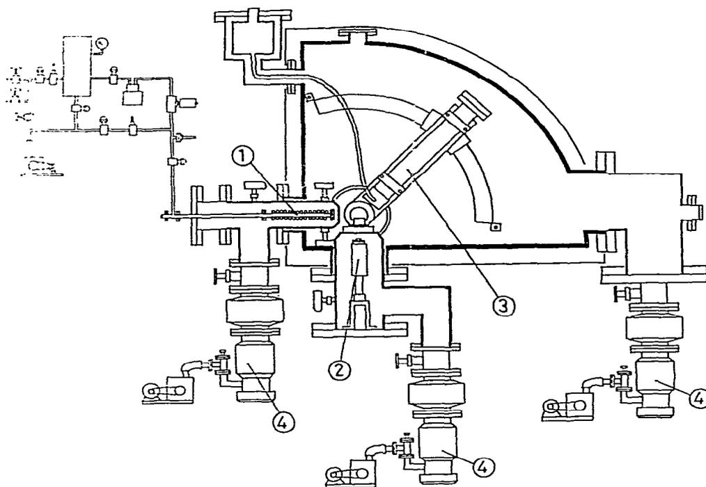
Fig. 1. Experimental arrangement. 1. molecular beam source; 2. atomic beam source; 3. quadrupole mass filter; 4. vacuum system.
