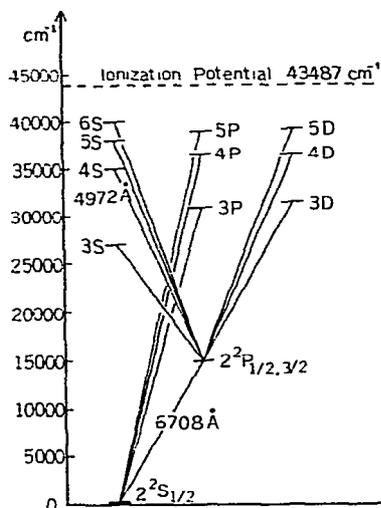
Fig. 2. Schematic energy diagram of lithium atom.
