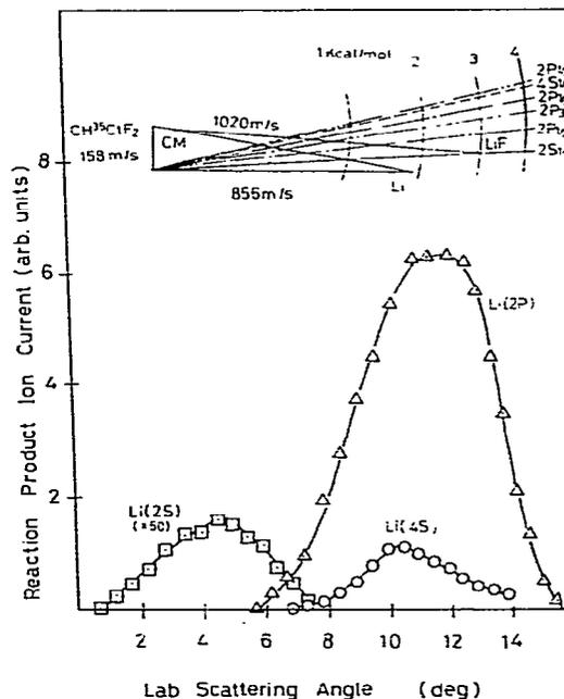
Fig. 3. Angular distribution of the isotopically non-selective reaction product LiF produced by the reaction of  $\text{CHCl}_2\text{F}$  with the lithium atom excited with a broadband laser. The molecular isotope detected is  $\text{LiF}$ ; the states used are the ground state (2S) and the excited states (2P and 4S).
