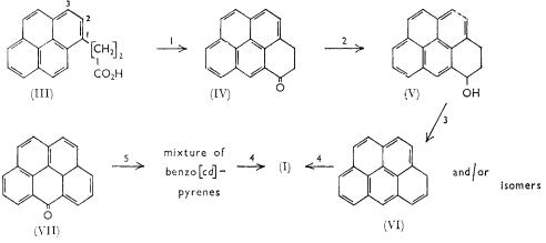
Reagents: I, HF. 2, LiAIH<sub>4</sub>. 3, HCI-CH<sub>3</sub>CO<sub>2</sub>H. 4, o-Chloranil-HCIO<sub>4</sub>. 5, LiAIH<sub>4</sub>-AICI<sub>3</sub>.
