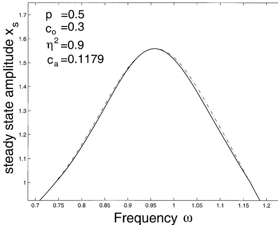
**FIG. 7. Frequency Response Curves of Bilinear Hysteretic Oscillator (Solid Curve) and Bilinear Nonhysteretic Oscillator (Dotted-Dashed Curve) with Corresponding Value of  $c_a$  for Resonant Amplitude Match**
