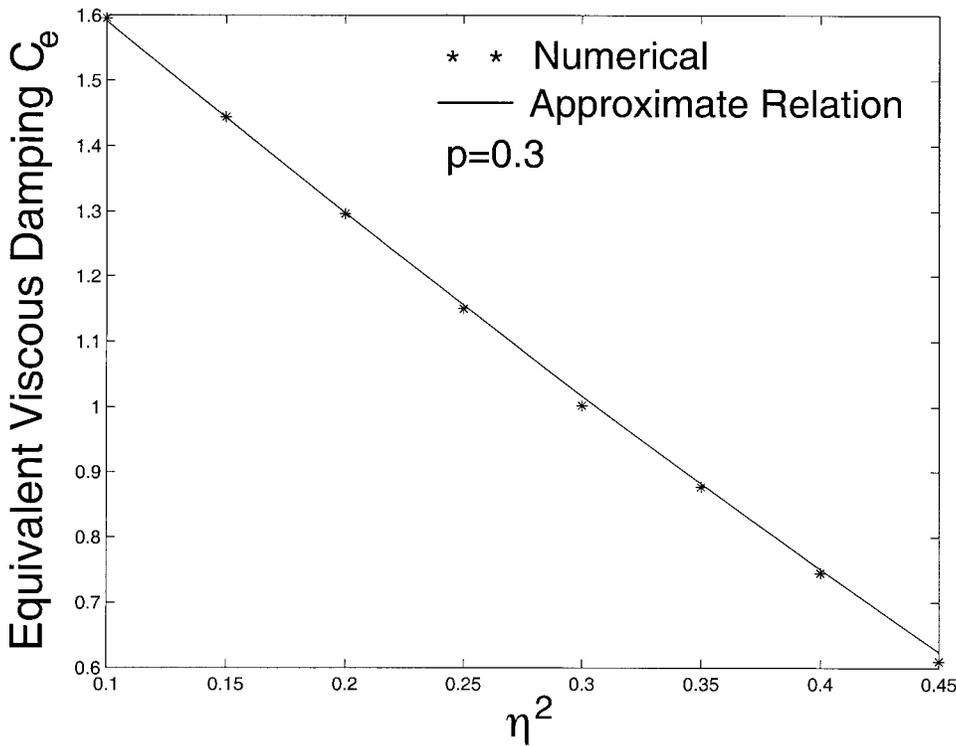
FIG. 10. Comparison of Approximate Relation between  $C_e$  and  $\eta^2$  with Values Obtained Numerically
