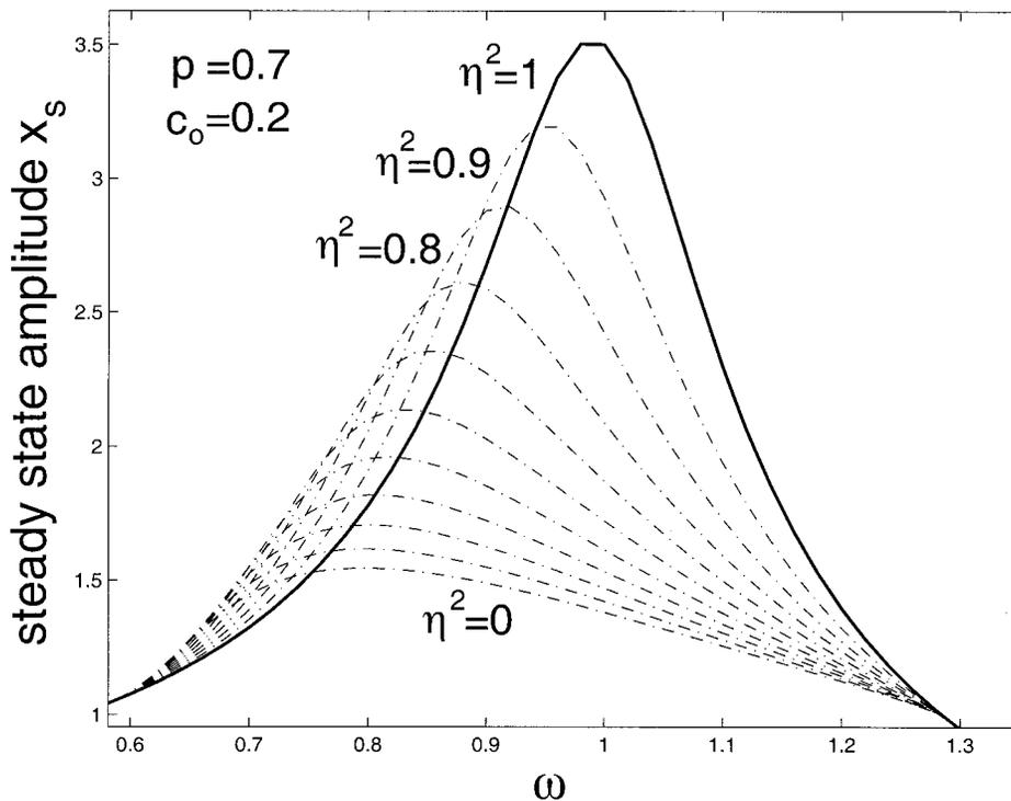
FIG. 5. Frequency Response Curves for Values of  $p$  and  $c_0$  outside Region I
