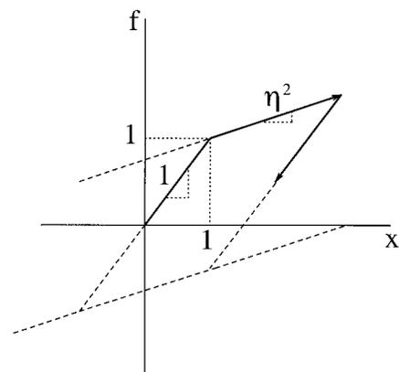
FIG. 1. Force Deflection Diagram for Bilinear Hysteresis
