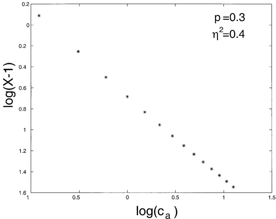
FIG. 9. Logarithmic Plot of  $X - 1$  against  $c_a$  for Bilinear Nonhysteretic Oscillator
