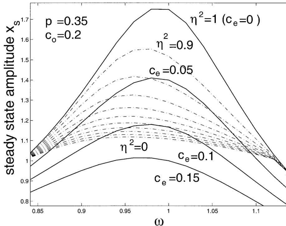
FIG. 6. Frequency Response Curves for Different Values of  $\eta^2$  (Dotted-Dashed Curve) and  $c_e$  (Solid Curve) for Same  $p$  and  $c_0$
