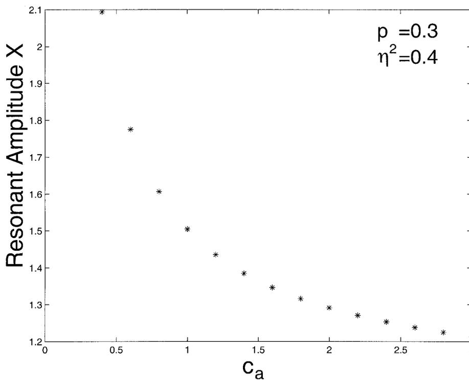
**FIG. 8. Variation of  $X$  against  $c_a$  for Given Values of  $p$  and  $\eta^2$  for Bilinear Nonhysteretic Oscillator**
