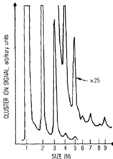
Fig. 2. Mass spectrum of  $\text{Rb}_N^+$  ( $N=1 \rightarrow 9$ ) generated by Rb liquid metal ion source (LMIS). For emission currents larger than  $60 \mu\text{A}$  copious production of clusters up to  $N=50$  is observed. The Rb heat pipe is at  $25^\circ\text{C}$ .
