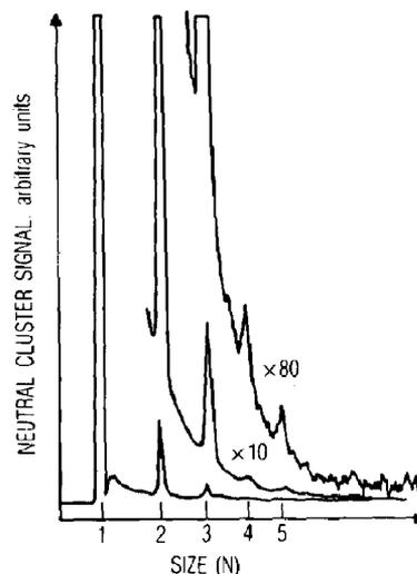
Fig. 3. Mass spectrum of neutral clusters ( $\text{Rb}_N$ ) emerging from the Rb heat pipe–charge exchange region which is heated to about  $200^\circ\text{C}$ . The large attenuation of the  $\text{Rb}_N^+$  beam is measured with CEM1 and the neutralized clusters are detected directly with CEM2. The aperture in front of CEM2 limits the acceptance angle.
