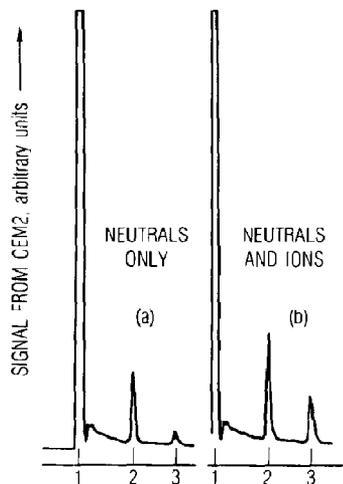
Fig. 4. Comparison of the signals with and without deflecting off the cluster ions. From this type of data we measure the charge exchange cross sections.
