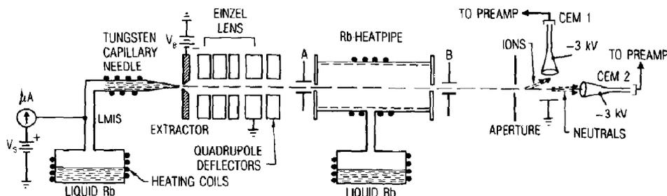
Fig. 1. Experimental apparatus used in the study of charge exchange of  $\text{Rb}_N^+$  with Rb atomic vapor. The aperture in front of the detector (CEM2) limits the acceptance angle.
