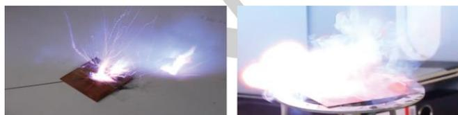
**Figure 15** Moment of deflagration of compound **7** during the hot needle test (left) and hot plate test (right).
