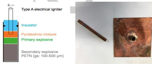
**Figure 16** Schematic test setup (left); copper shell and plate before the initiation capability test (right).
