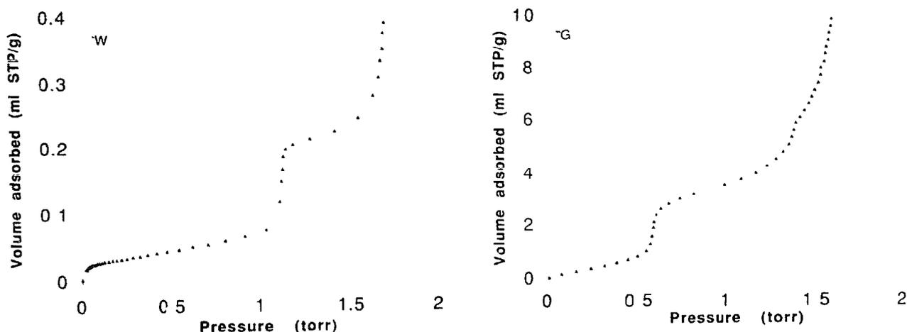
Fig. 3. Adsorption isotherms for krypton on LiF powders at 77.3 K for LiF "W" and LiF "G", saturating pressure: 1.73 Torr.
