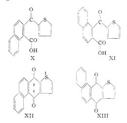
Pure samples of XII and XIII were prepared from X and XI, respectively, by reduction to the corresponding thenylnaphthoic acids, cyclization to acetoxybenzthiophanthrene derivatives, and oxidation to XII and XIII.
