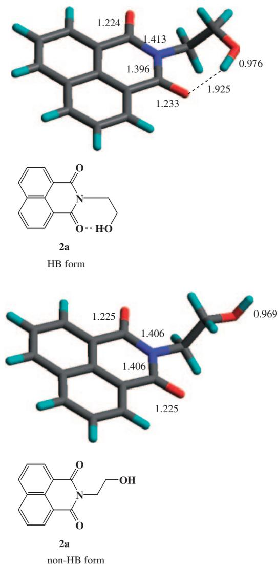
**Figure 4.** Optimized hydrogen bonding geometry (HB form, total energy =  $-262.91533$  kcal mol $^{-1}$ ) and non-hydrogen bonding geometry (non-HB form, total energy =  $-262.72322$  kcal mol $^{-1}$ ) for naphthalimide **2a** calculated using RB3LYP/6-31+G(d) (lengths in Å).
