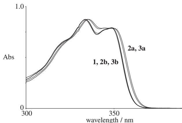
**Figure 1.** UV spectra of naphthalimides **1–3** (0.075 mM) in dichloromethane.
