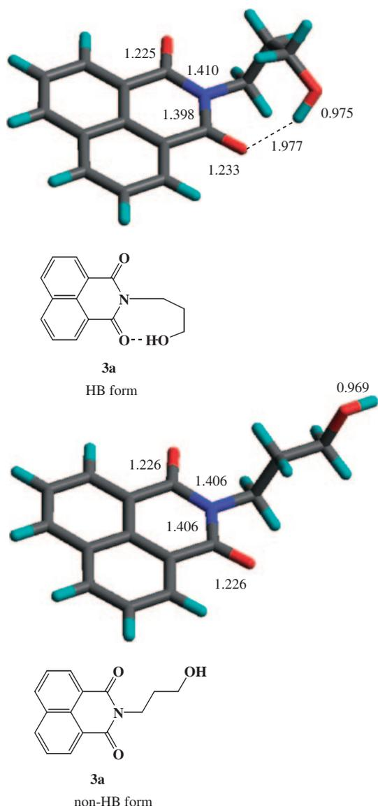
**Figure 5.** Optimized hydrogen bonding geometry (HB form, total energy =  $-287.32382$  kcal mol $^{-1}$ ) and non-hydrogen bonding geometry (non-HB form, total energy =  $-286.80799$  kcal mol $^{-1}$ ) for naphthalimides **3a** calculated using RB3LYP/6-31+G(d) (lengths in Å).
