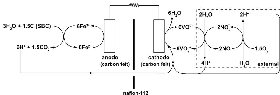
**Figure 1.** Schematic representation of the coal fuel cell which simplifies the stoichiometry of the reaction between SBC and  $\text{Fe}^{\text{III}}$  ions given in Equation (2).
