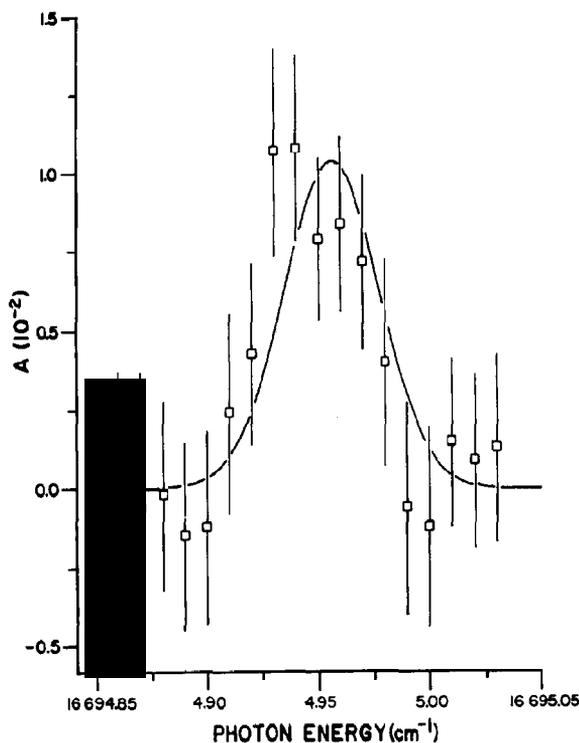
Fig. 4. Photo-assisted fragmentation spectrum of the  $H_3$  radical. Vertical lines represent one standard deviation error bars. The smooth curve represents a least-squares fit of the data to a Gaussian function with a  $0.05 \text{ cm}^{-1}$  full width at half maximum.
