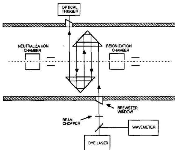
Fig. 3. Partial schematic of the apparatus depicting modifications for obtaining photo-assisted fragmentation (PAF) spectra.
