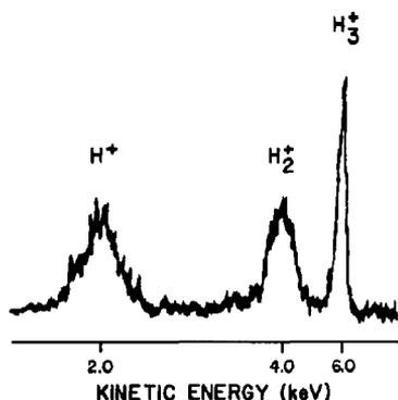
Fig. 2. Neutralization–reionization mass spectra of  $H_3^+$  obtained using K as the neutralization target and  $N_2$  as the reionization target.
