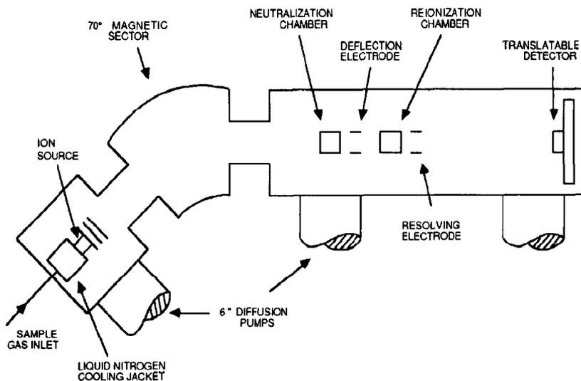
Fig. 1. Schematic of the apparatus configured to obtain non-optical neutralization-reionization mass spectra.
