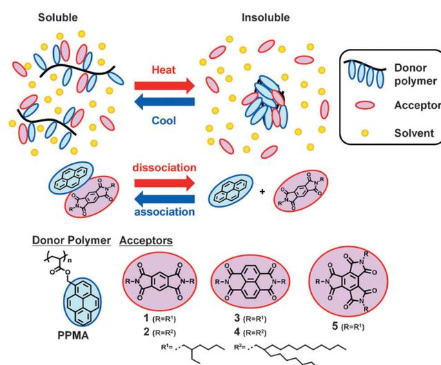
**Figure 1.** Concept of the LCST behavior of supramolecular complexes as caused by a CT interaction, and structure of the effectors studied and the polymer PPMA, which contains pyrene groups as donor moieties.
