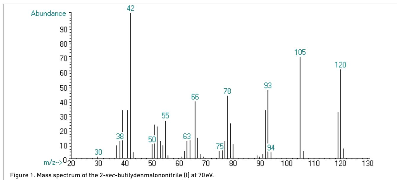
Figure 1. Mass spectrum of the 2-sec-butylidenmalononitrile (**I**) at 70 eV.
