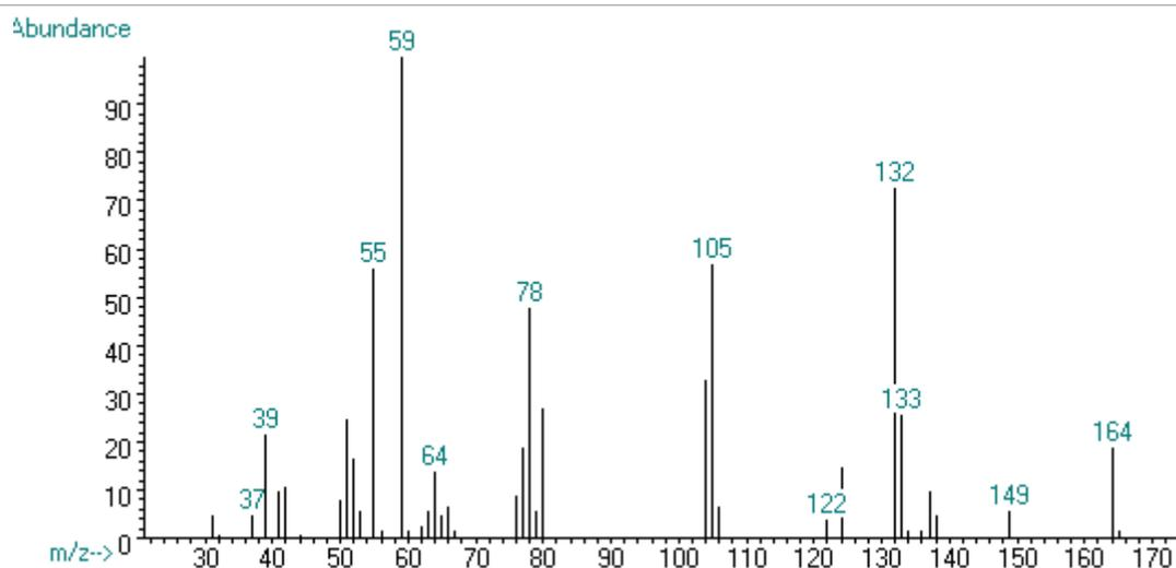
Figure 3. Mass spectrum of 4,4-dicyano-3-methyl-3-butenic methyl ester (III) at 70 eV.
