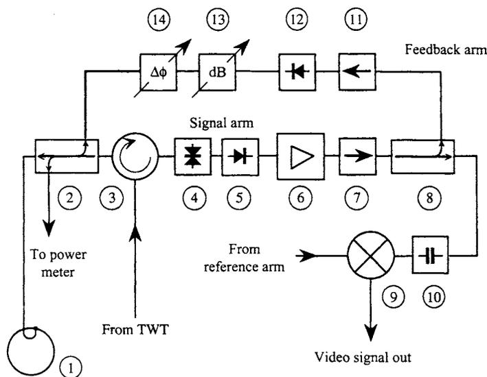
**Fig. 5.** Principal diagram of the modified S/C-band spin echo spectrometer used for the time-variable feedback experiments: (1)–(10) receiver (signal) arm, (11)–(14) additional (feedback) arm. (1) Resonator; (2) directional coupler (–6 dB); (3) circulator; (4, 5) receiver protection pin-switches; (6) low-noise input amplifier (+20 dB); (7) isolator; (8) directional coupler (–6 dB); (9) mixer; (10) DC block; (11) isolator; (12) feedback timing pin-switch; (13) attenuator; (14) phase shifter.
