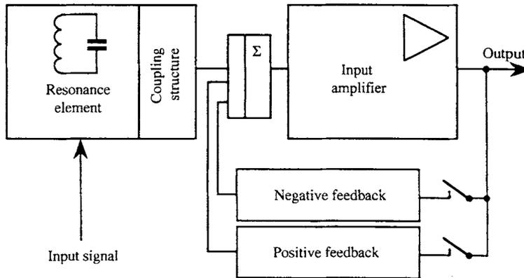
Fig. 1. Principal block diagram of the magnetic resonance receiver comprising the resonance element with coupling structure and input amplifier with two-branch feedback system controlled by switches.
