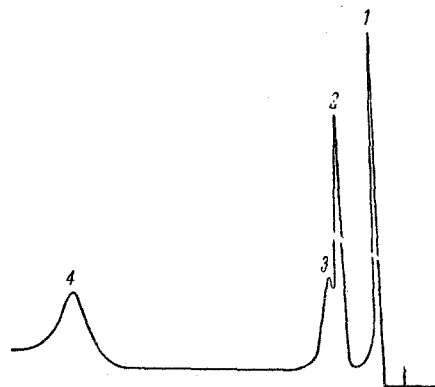
Fig. 2. Chromatogram of the hydrolyzate of malonaldehyde bis(diethyl acetal). Hydrolysis conditions: (I): H_2O = 1 : 1 ; 3% of p-CH_3C_6H_4SO_3H in aqueous phase; 100°; 5 min. Chromatography conditions: 100°; consumption of helium 80 ml/min: peak (1), alcohol; peak (2), C_2H_5OCH=CHCHO ; peak (3), (C_2H_5O)_2CHCH_2CHO ; peak (4), (C_2H_5O)_2CHCH_2CH(OC_2H_5)_2 .
