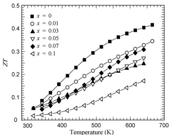
Fig. 4. Temperature dependences of the dimensionless figure of merit,  $ZT$ , for  $\text{Mg}_{2-x}\text{Ca}_x\text{Si}$ .
