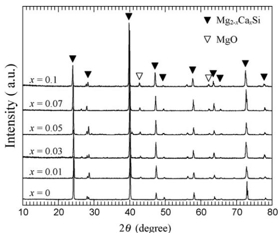
Fig. 1. XRD patterns for  $\text{Mg}_{2-x}\text{Ca}_x\text{Si}$  compounds.
