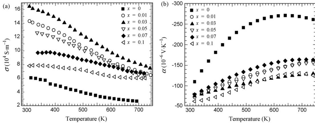
Fig. 2. Temperature dependences of electrical conductivity  $\sigma$  (a) and Seebeck coefficient  $\alpha$  (b) for  $\text{Mg}_{2-x}\text{Ca}_x\text{Si}$ .
