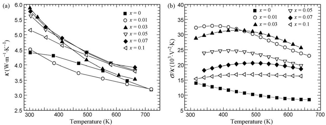
Fig. 3. Temperature dependences of thermal conductivity  $\kappa$  (a) and the electron- to phonon-conduction ratio  $\sigma/\kappa$  (b) for  $\text{Mg}_{2-x}\text{Ca}_x\text{Si}$ .
