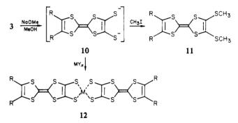
which can then be treated with methyl iodide to provide unsymmetrically substituted TTF derivatives (11,  $R = CO_2CH_3$ ). Alternately, treatment of 10 with transition-metal salts yielded a wide variety of novel metal dithiolene derivatives (12) which incorporate TTF as conjugated ligands.<sup>8</sup>
