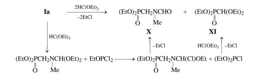
The presented reaction scheme agrees with data in [6]. Amides **II–IV** containing a three-coordinate phosphorus atom were used by us to prepare novel four-coordinate phosphorus compounds with a PCH<sub>2</sub>NP fragment.
