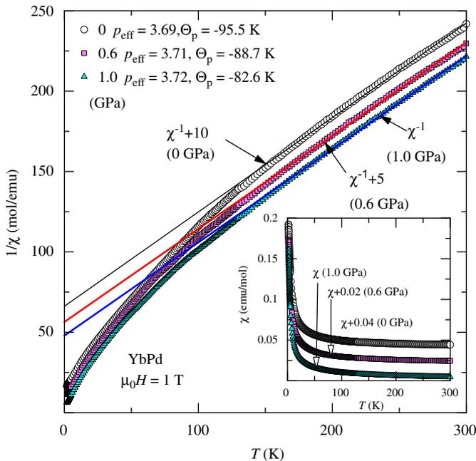
Fig. 1. Temperature dependence of inverse magnetic susceptibility of YbPd at various pressures. The solid line shows a Curie–Weiss law. The effective Bohr magneton number,  $\mu_{\text{eff}}$ , and Weiss temperature,  $\Theta_p$ , estimated from the Curie–Weiss law, are indicated for each pressure. The inset shows magnetic susceptibility as a function of temperature.
