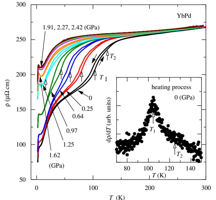
Fig. 2. Temperature dependence of the electrical resistivity of YbPd under high pressure. The white arrows show phase transition temperatures,  $T_1$  and  $T_2$ . The inset exhibits  $d\rho/dT$  as a function of temperature. We define  $T_1$  as a peak position.
