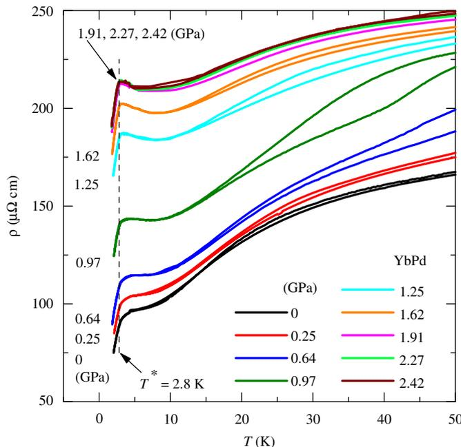
**Fig. 4.** Temperature dependence of the electrical resistivity of YbPd under high pressures in the temperature range between 2 and 50 K. At around 2.8 K, a bend or a peak is observed at all pressures studied.
