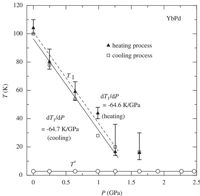
**Fig. 3.** Pressure dependence of the transition temperature  $T_1$  measured during heating and cooling. The error bar is shown only for heating process. The rate of  $dT_1/dP$  is estimated to be  $\sim -65$  K/GPa. The  $T^*$ , which would be associated with magnetic ordering, is also plotted as a function of pressure.
