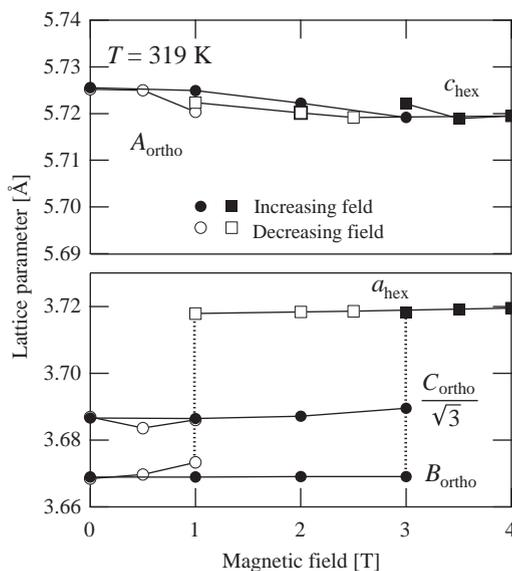
Fig. 6. Magnetic field dependence of lattice parameters of MnAs at 319 K. Closed and open symbols show the lattice parameters for the increasing and decreasing field process, respectively. Dotted lines denote the two-phase coexistence of the NiAs-type and MnP-type at 3 T for the increasing and at 1 T for decreasing field, respectively.
