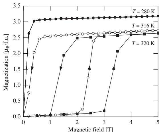
Fig. 1. Magnetization curves around  $T_C$ . The inset shows the temperature dependence of magnetization at 0.01 T.
