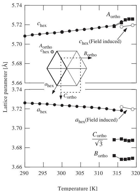
Fig. 5. Temperature dependence of lattice parameters of MnAs. The lattice parameters of the field-induced hexagonal structure at 4 T is also plotted as open circles.
