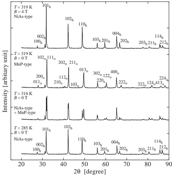
Fig. 2. X-ray diffraction profiles of MnAs at several temperatures around  $T_C$ . The Miller indices are represented as  $hkl_o$  for the orthorhombic type and  $hkl_h$  for the hexagonal type structure. Some indices of the unresolved multiplets are omitted to display.
