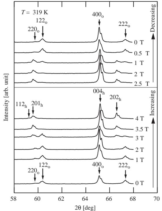
Fig. 4. X-ray diffraction profiles of MnAs at 319 K in magnetic fields up to 4 T. The lower and upper panels show the profiles with increasing and decreasing magnetic fields, respectively.
