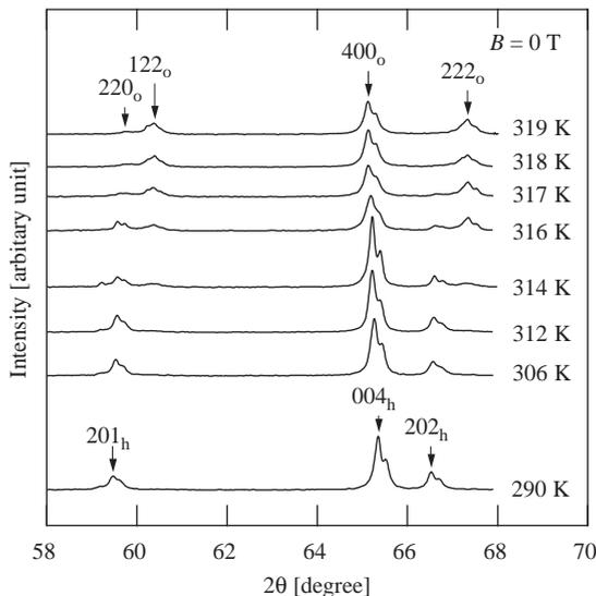
Fig. 3. X-ray diffraction profiles of MnAs at several temperatures at 0 T around  $T_C$ .
