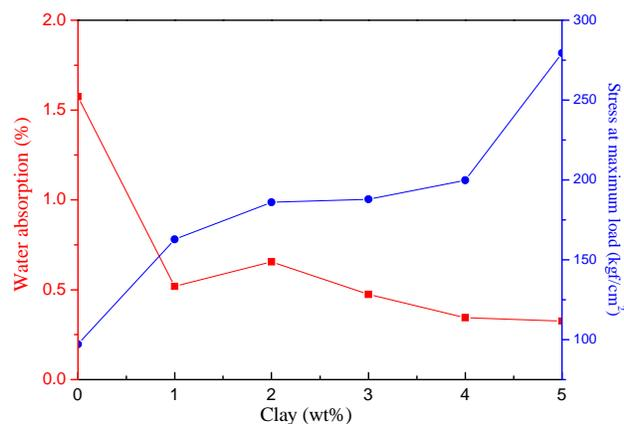
Fig. (8). Influence of MMT content on water absorption and tensile strength of films.
