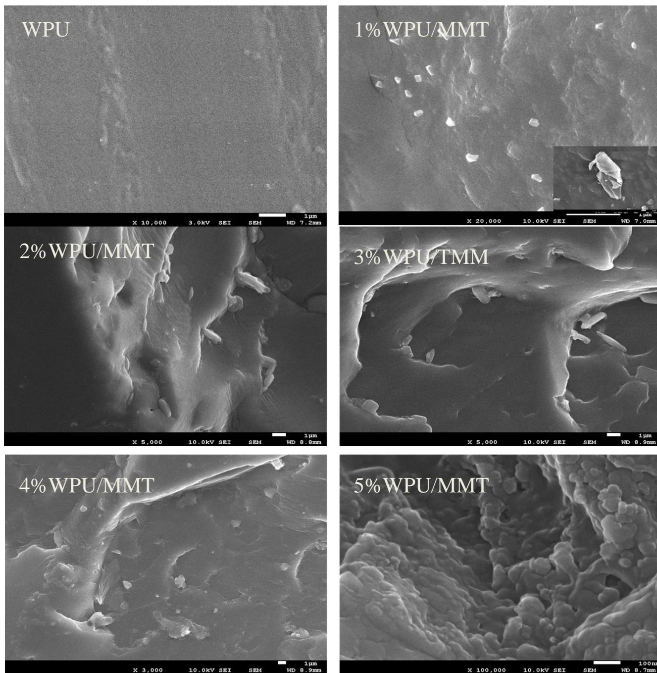
Fig. (6). SEM pictures of WPU and WPU/MMT composites.
