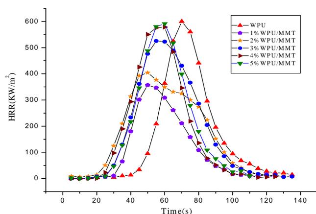
Fig. (9). HRR curves of WPU and MMT/WPU composites.
