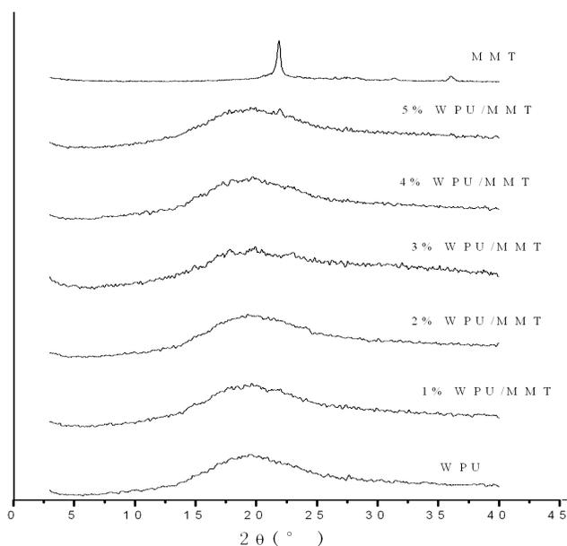
**Fig. (5).** XRD spectra of WPU and WPU/MMT composite films.
