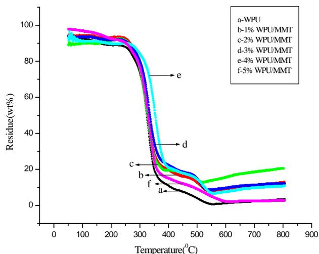
Fig. (7). TGA thermographs of WPU and WPU/MMT films.
