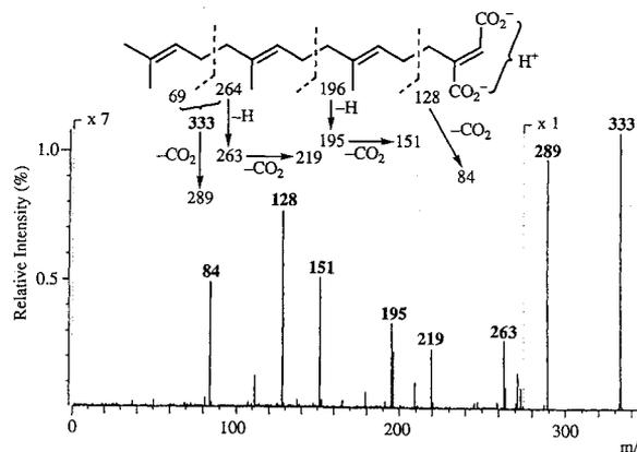
Fig. 2b. MS/MS fragmentation pattern of  $(M-2H+3Li)^+$  ions ( $m/z$  353) in the positive-ion FAB-MS spectrum.
