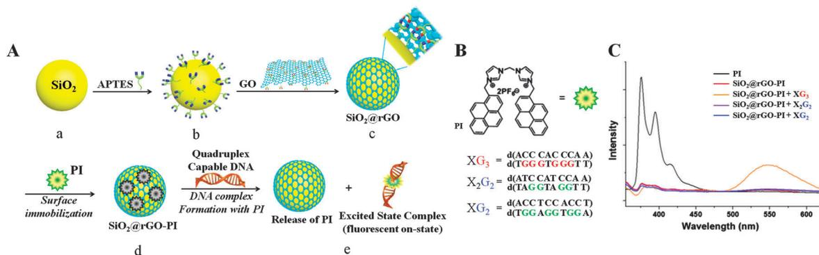
**Fig. 1** (A) Schematic of the preparation method for SiO<sub>2</sub>@rGO-PI; (a) SiO<sub>2</sub> particles, (b) amino group functionalized SiO<sub>2</sub> particles, (c) rGO wrapped SiO<sub>2</sub> particles, (d) PI adsorbed onto SiO<sub>2</sub>@rGO and (e) PI released from SiO<sub>2</sub>@rGO. (B) Chemical structure of PI and the various DNA used in this study. (C) Fluorescence spectra of PI, SiO<sub>2</sub>@rGO-PI, and also SiO<sub>2</sub>@rGO-PI in the presence of various DNA.
