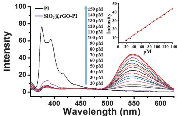
**Fig. 3** Fluorescence spectra originating from PI and SiO<sub>2</sub>@rGO-PI upon incubation with XG<sub>3</sub> DNA (0–150 pM). Inset: 550 nm fluorescence intensity as a function of picomolar XG<sub>3</sub> concentration (pM) upon addition to SiO<sub>2</sub>@rGO-PI.
