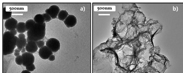
**Fig. 2** (a) TEM image of SiO<sub>2</sub>@rGO. (b) TEM image of SiO<sub>2</sub>@rGO after washing with basic solution (0.1 M NaOH).
