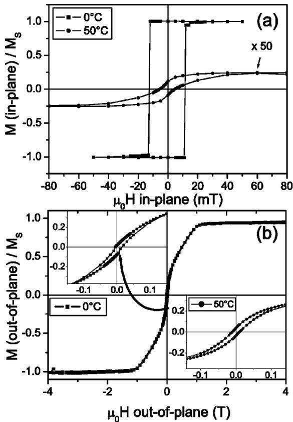
FIG. 2. Magnetic hysteresis measurements of a 60 nm MnAs/GaAs(001) film at 0 °C and 50 °C. The external field is applied (a) in the film plane along the *a* axis and (b) out-of-plane. Note, that the in-plane hysteresis at 50 °C is normalized to the saturation magnetization at  $T=0$  °C ( $M_S = 0.65$  MA/m) and magnified by a factor of 50. The two insets of (b) enlarge the low-field range revealing clear out-of-plane hysteretic behavior.
