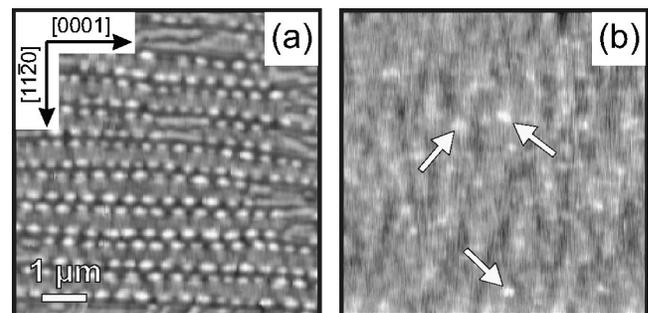
FIG. 1. MFM images of a 180 nm MnAs/GaAs(001) film (see Ref. 13) at (a) 15 °C and (b) 41 °C. (a) shows the coexistence of the ferromagnetic  $\alpha$ - and the paramagnetic  $\beta$ -phase; the  $\alpha$ -phase is demagnetized thus showing a zigzag-shaped domain pattern of the  $\alpha$ -stripes. In image (b), some residual contrast of small isolated dots is visible (arrows).
