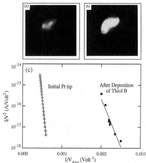
**Figure 4.** (a, b) Field emission patterns from a Pt (100) after deposition of thiol B (550, 600 V). (c) Fowler–Nordheim plots for the emission from the cleaned Pt (100) and after immersion in thiol B.
