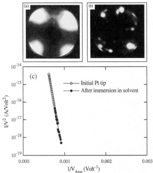
**Figure 2.** Field emission patterns from (a) Pt (100) (1500 V) and (b) Pt (100) after being immersed in the dichloromethane for 18 h and then reinserted in the UHV (1400 V). (c) Fowler–Nordheim plots for the emission from the cleaned Pt (100) and after immersion in the solvent.
