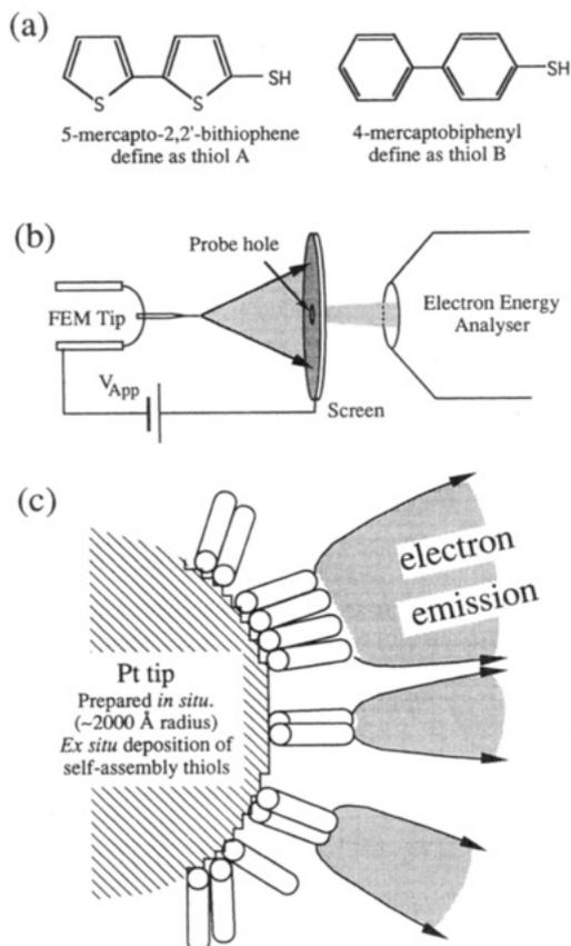
**Figure 1.** (a) Organic thiols used in the experiment. (b) Experimental setup for the measurement of the electron energy distributions. Not shown are the mechanical and electrical deflections which allow selection of the emission zone that passes through the probe hole. (c) Schematic depiction of the field emission from a tip with adsorbed thiol molecules.
