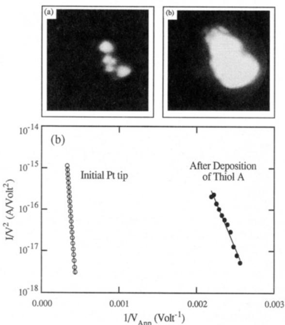
**Figure 3.** (a, b) Field emission patterns from a Pt (100) after deposition of thiol A (400, 500 V). The voltages were increased from (a) to (b) to show that a relatively large area of the tip has been affected by exposure to the organics. (c) Fowler–Nordheim plots for the emission from the cleaned Pt (100) and after immersion in the thiol A.
