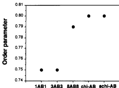
**Figure 10.** Order parameters of azobenzene derivatives doped in FLC 1. The concentration of azobenzene was 3 mol %. Measurements were performed at 55 °C.
