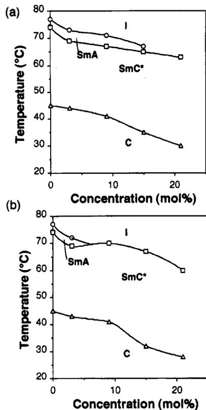
**Figure 7.** Phase diagram of the chi-AB/FLC 1 mixture: (a) before irradiation; (b) after irradiation at 366 nm. The concentration of azobenzene was 3 mol %, and the degree of isomerization after irradiation was estimated as ~80%.
