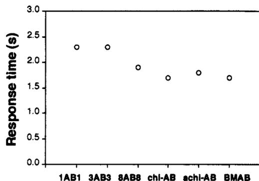
**Figure 3.** Response times of photochemical switching of polarization in azobenzene derivatives/FLC 1 mixtures induced by steady-state irradiation. Irradiation was performed at 366 nm with a light intensity of 36 mW/cm<sup>2</sup>.
