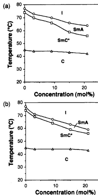
**Figure 9.** Phase diagram of the BMAB/FLC 1 mixture: (a) before irradiation; (b) after irradiation at 366 nm. The concentration of azobenzene was 3 mol %, and the degree of isomerization after irradiation was estimated as ~80%.
