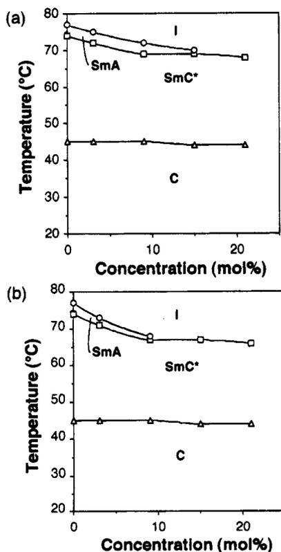
**Figure 8.** Phase diagram of the achi-AB/FLC 1 mixture: (a) before irradiation; (b) after irradiation at 366 nm. The concentration of azobenzene was 3 mol %, and the degree of isomerization after irradiation was estimated as ~80%.
