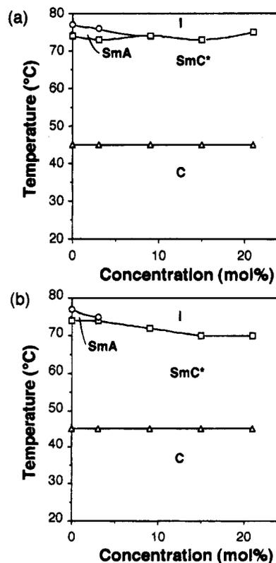
**Figure 6.** Phase diagram of the 8AB8/FLC 1 mixture: (a) before irradiation; (b) after irradiation at 366 nm. The concentration of azobenzene was 3 mol %, and the degree of isomerization after irradiation was estimated as  $\sim 80\%$ .
