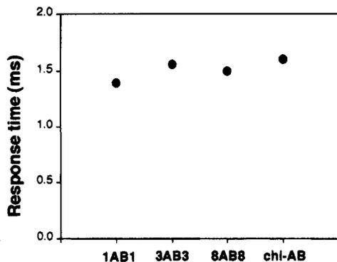
**Figure 2.** Response times of photochemical switching of polarization in azobenzene derivatives/FLC 1 mixtures induced by pulsed laser irradiation. Irradiation was performed at 355 nm with an intensity of 100 mJ/cm<sup>2</sup>.
