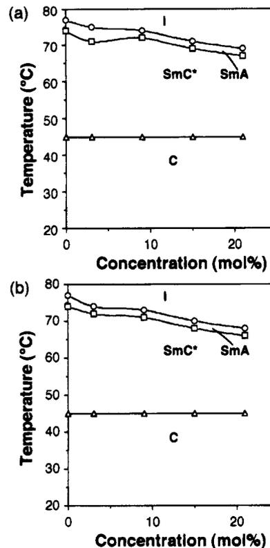
**Figure 5.** Phase diagram of the 3AB3/FLC 1 mixture: (a) before irradiation; (b) after irradiation at 366 nm. The concentration of azobenzene was 3 mol %, and the degree of isomerization after irradiation was estimated as  $\sim 80\%$ .
