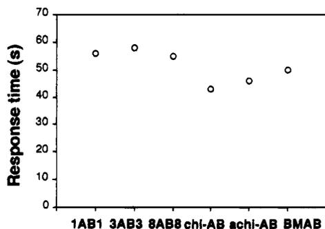
**Figure 11.** Response times of the photochemical SmC\*–SmA phase transition in the azobenzene derivative/FLC 1 mixtures induced by steady-state irradiation at 366 nm.  $T = T_c - 1$  °C.
