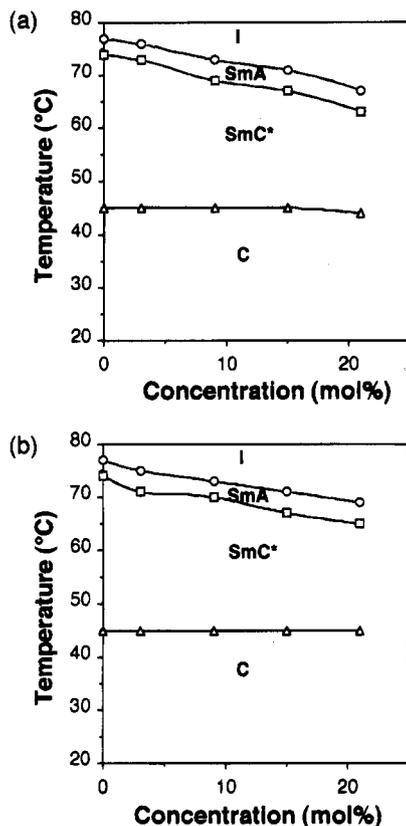
**Figure 4.** Phase diagram of the 1AB1/FLC 1 mixture: (a) before irradiation; (b) after irradiation at 366 nm. The concentration of azobenzene was 3 mol %, and the degree of isomerization after irradiation was estimated as  $\sim 80\%$ .
