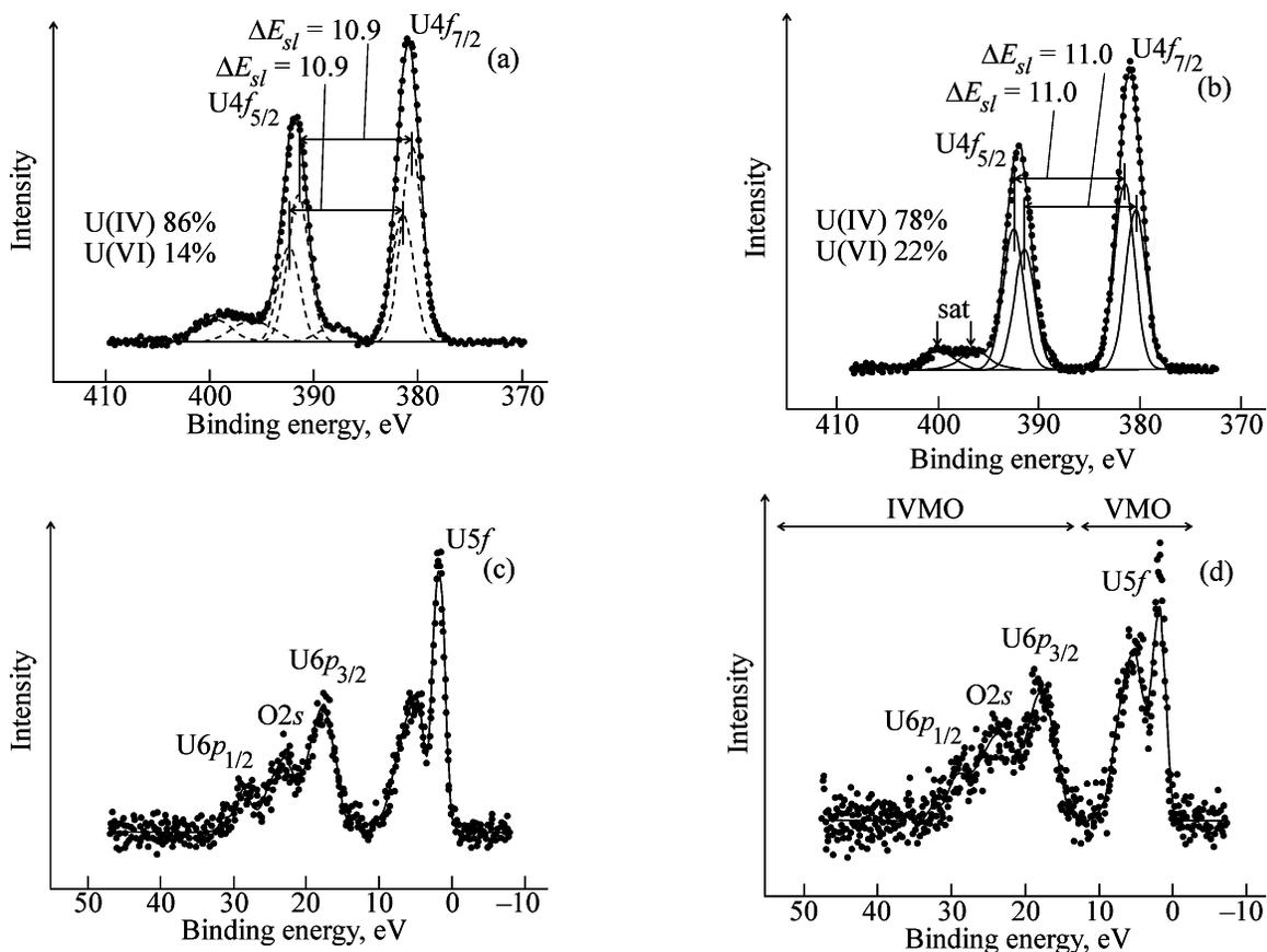
**Fig. 3.** X-ray photoelectron spectra of (a, b)  $U4f$  electrons and (c, d) valence electrons of  $UO_{2+x}$  samples kept at pH (a, c) 2.54 and (b, d) 7.04. The bands were resolved in the approximation that the samples contain only U(IV) and U(VI).
