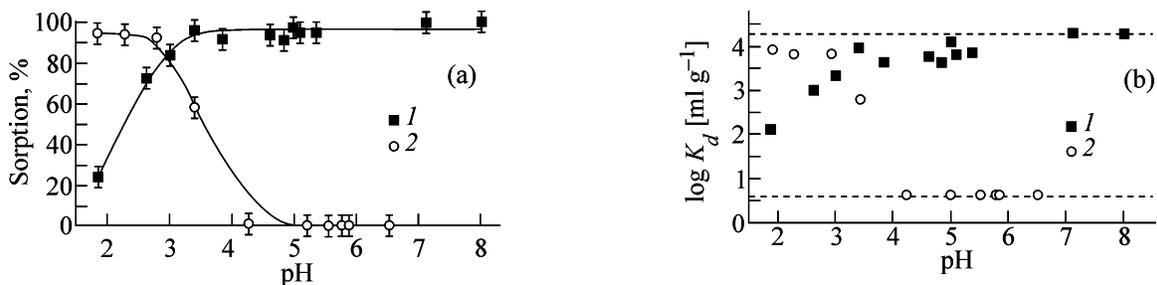
**Fig. 4.** (a) Fraction of (1) Tc(IV) and (2) Tc(VII) sorbed on  $UO_{2+x}$  and (b) logarithm of distribution coefficients of these species as functions of pH.
