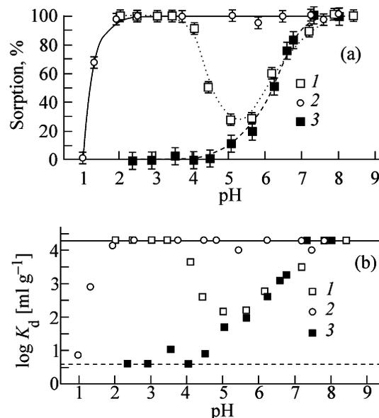
**Fig. 1.** (a) Fraction of (1) Np(V) and (2) Th(IV) sorbed on  $\text{UO}_{2+x}$  and (3) fraction of Np(V) sorbed on  $\text{ThO}_2$ , and (b) logarithm of distribution coefficients of these radionuclides, as functions of pH.
