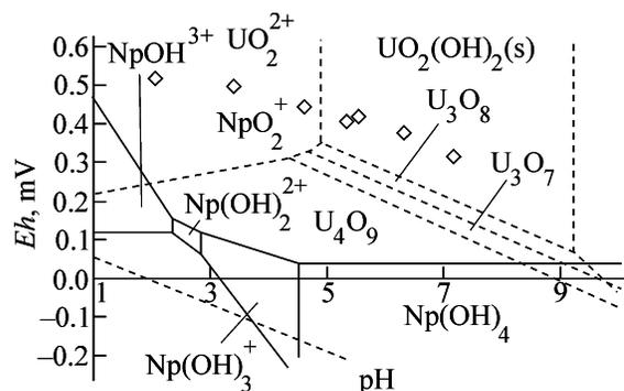
**Fig. 2.** Pourbaix diagram for Np (continuous line) and U [17] (dashed line). The Eh potential is given vs. standard hydrogen electrode. Points denote the conditions of sorption experiments.
