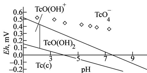
**Fig. 5.** Pourbaix diagram for Tc. The  $Eh$  potential is given vs. a standard hydrogen electrode. Points denote the conditions of sorption experiments.
