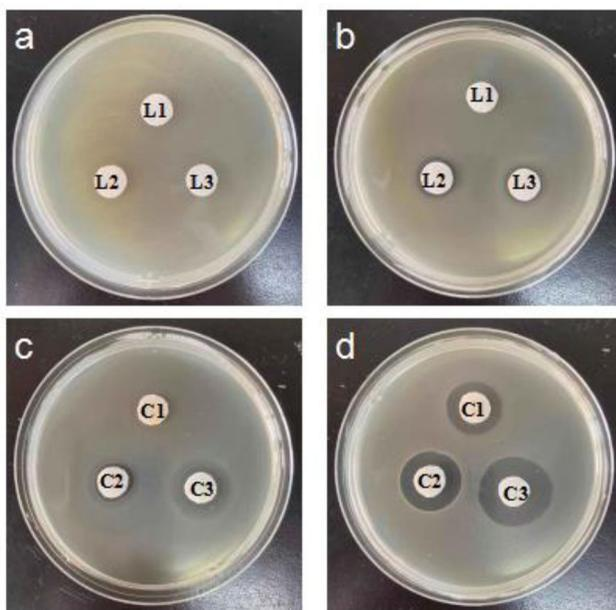
**Figure 5.** Zone of inhibition against microorganisms (a, c) *S. aureus*; (b, d) *E. coli*.
