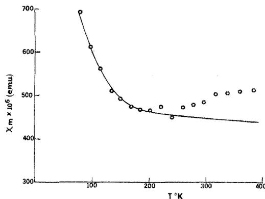
Figure 6. Magnetic susceptibility vs. temperature for DiB-N-MPClO<sub>4</sub>: points, experimental; line, calculated from Ising model for  $J = 0.036$  eV, assuming 15% of a paramagnetic impurity.
