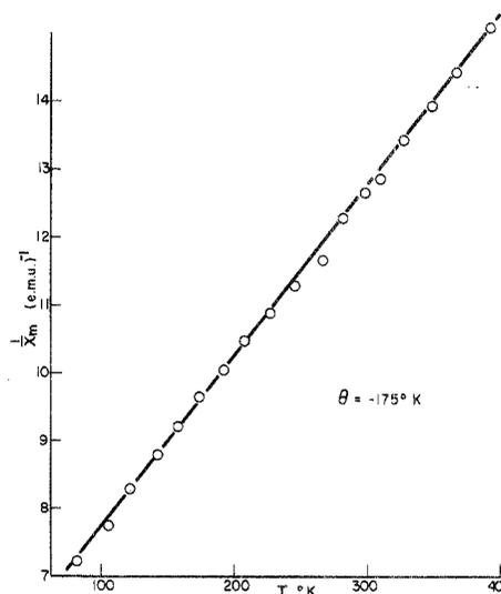
Figure 3. Reciprocal magnetic susceptibility vs. temperature for 10-MPClO<sub>4</sub>.
