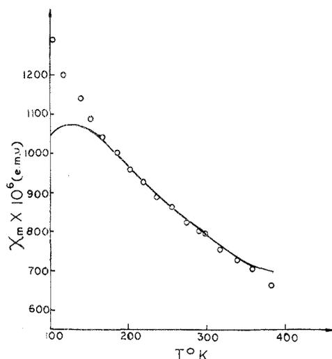
Figure 5. Magnetic susceptibility vs. temperature for 10-MPClO<sub>4</sub>: solid line, calculated from Ising model equation using  $J = 0.011$  eV; points, experimental.
