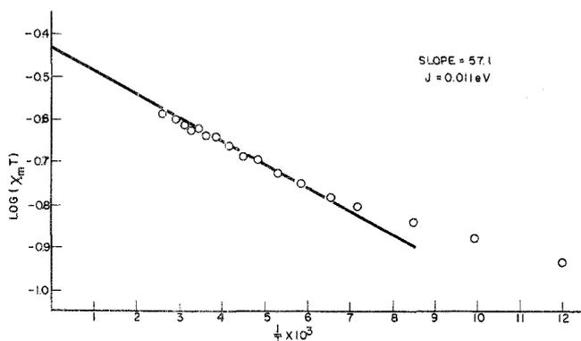
Figure 4. Insing model plot for 10-MPClO<sub>4</sub>.
