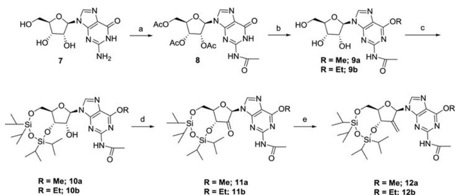
**Scheme 1.** Reagents and conditions. (a) acetic anhydride, pyridine, 70°C; 92%; (b) *i.* DIAD, EtOH or MeOH, dioxane. *ii.* Ammonium hydroxide, methanol; **9a**: 93% over two steps, **9b**: 86% over two steps.; (c) tetraisopropylidisiloxanedichloride pyridine; **10a**: 97%, **10b**: 82%; (d) Dess-Martin periodinane, CH<sub>2</sub>Cl<sub>2</sub>; **11a**: 65%, **11b**: 78%; (e) methyltriphenylphosphonium bromide, potassium hexamethyldisilazide, THF; **12a**: 52%, **12b**: 66%.
