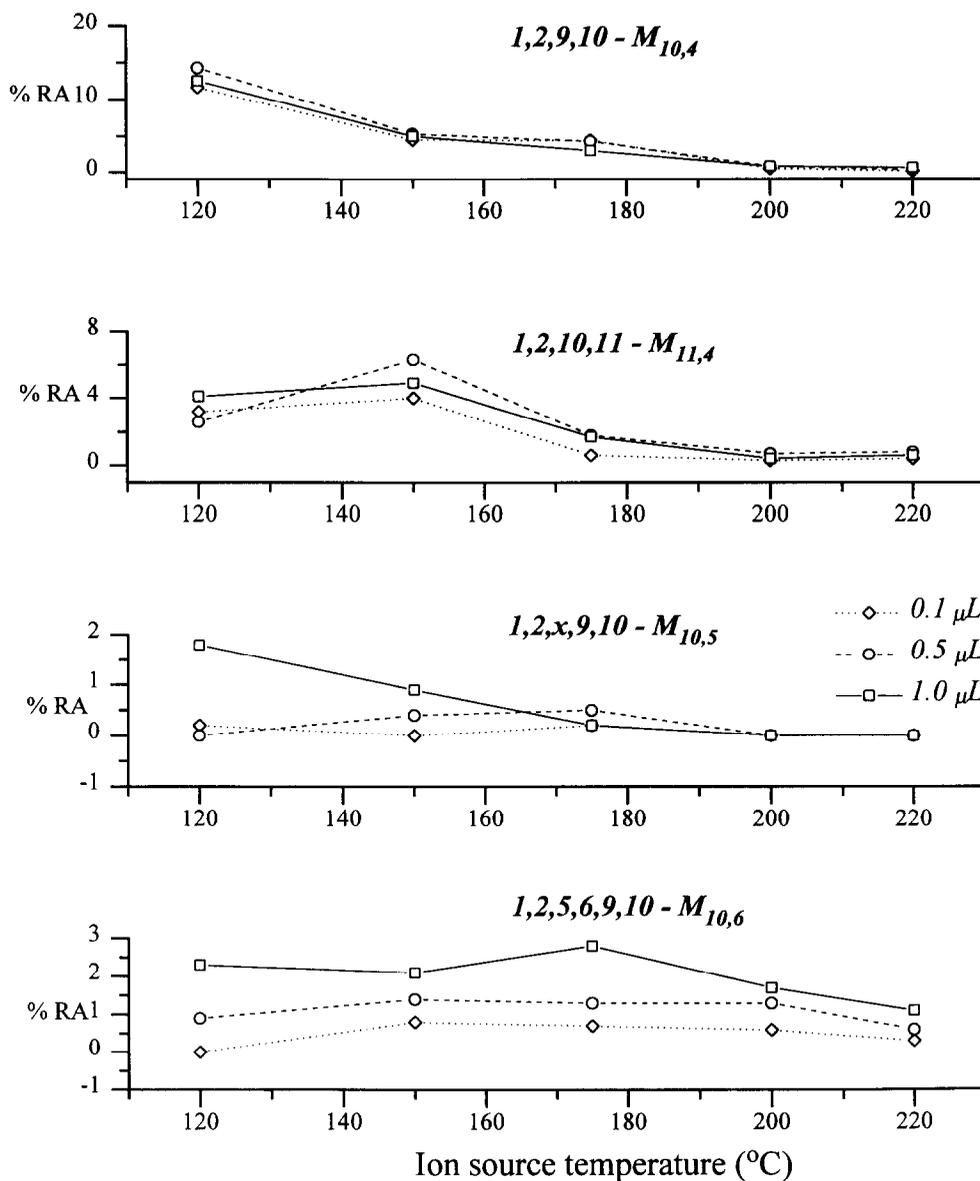
Figure 5. Effect of ion source temperature and volume of injected solution (see text) on the relative abundance of the  $[M + Cl]^-$  ion.
