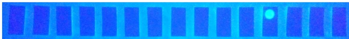
**Fig. 7.** Images of test papers for the selectivity of  $\text{Cr}^{3+}$  upon addition of 10 mM various metal ions (From left to right, the metal ions used were only **1**,  $\text{K}^+$ ,  $\text{Ca}^{2+}$ ,  $\text{Na}^+$ ,  $\text{Mg}^{2+}$ ,  $\text{Al}^{3+}$ ,  $\text{Zn}^{2+}$ ,  $\text{Co}^{2+}$ ,  $\text{Ni}^{2+}$ ,  $\text{Pb}^{2+}$ ,  $\text{Cu}^{2+}$ ,  $\text{Cr}^{3+}$ ,  $\text{Hg}^{2+}$ ,  $\text{Mn}^{2+}$  and  $\text{Cd}^{2+}$ ) under a UV lamp (365 nm).
