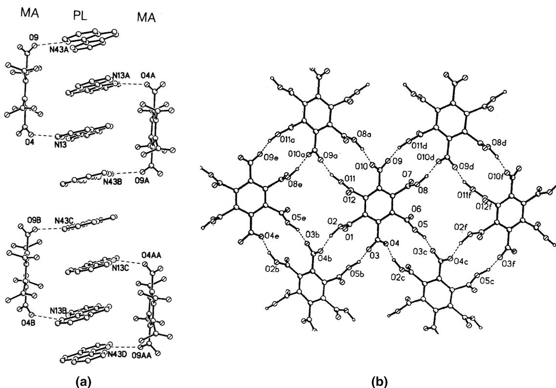
**Fig. 3** (a) An infinite interlocked assembly of MA–PL complex [1]. (b) Sheet structure of  $\text{MA}^{-2}$  in the MA–PL complex at right angles to (a). There are no water molecules in the crystal. Each  $\text{MA}^{-2}$  ion participates with 8 hydrogen bonds to form the sheet
