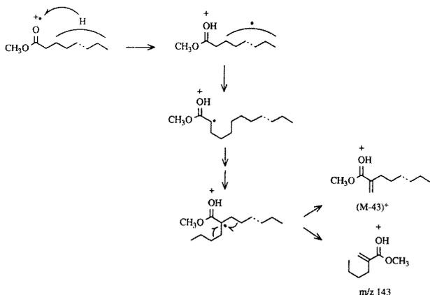
branched C atoms are regularly  $C_4$  units apart. For example, in the spectrum of methyl octacosanoate (Fig. 2), prominent peaks correspond to each other symmetrically
