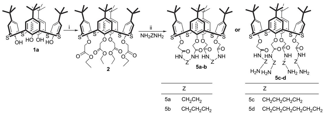
**Scheme 1.** (i) Na<sub>2</sub>CO<sub>3</sub>/BrCH<sub>2</sub>COOC<sub>2</sub>H<sub>5</sub>, acetone; (ii) toluene/methanol (1:1).
