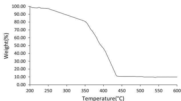
**Fig. 12** TGA diagram of calixarene-polyurethane composite at the temperature range 200–600 °C with heating rate of 10 °C  $\text{min}^{-1}$
