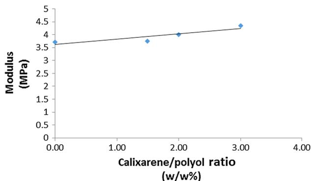
**Fig. 9** Modulus of calixarene-polyurethane composite versus the calixarene/polyol ratio
