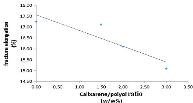
**Fig. 10** Fracture elongation of calixarene-polyurethane composite versus calixarene/polyol ratio
