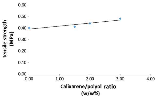
**Fig. 8** Tensile strength of calixarene-polyurethane composite versus calixarene/polyol ratio
