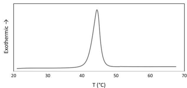
**Fig. 13** DSC heating thermograms of calixarene-polyurethane composite at the 5 °C  $\text{min}^{-1}$  scan rate
