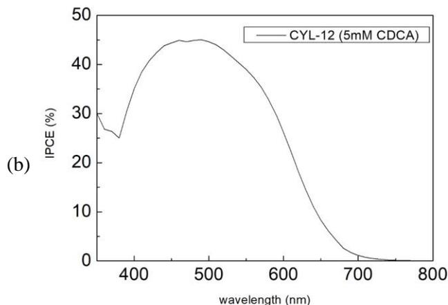
**Figure 2.** Photovoltaic characteristics of **CYL-12**: (a) photocurrent density vs. photovoltage; (b) incident photon-to-current conversion efficiency (IPCE)
