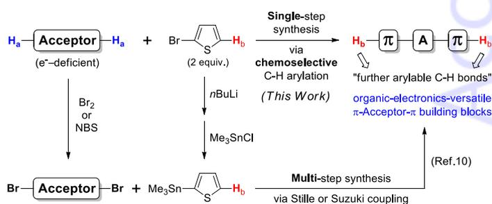
**Scheme 1.**  $\pi$ -acceptor- $\pi$  building blocks accessed by multi-step Stille coupling or single-step chemoselective C-H arylation.
