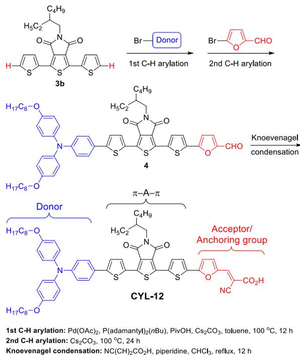
**Scheme 2.** Application of  $\pi$ -acceptor- $\pi$  building block (**3b**) in the facile synthesis of new organic sensitizer **CYL-12**.
