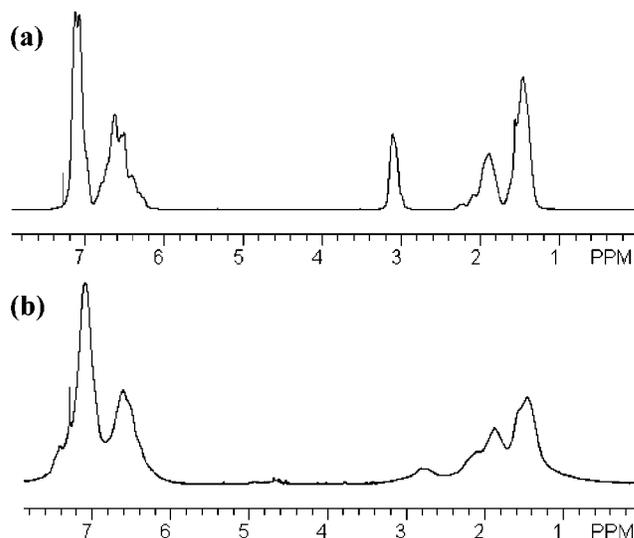
**Figure 2.** Comparison of <sup>1</sup>H NMR spectrum for (a) the starting linear polymer, **8**, 80/20 Sty/BCB,  $M_w = 95\,000$ , PDI = 1.12; and the resulting nanoparticle, **9**,  $M_w = 65\,000$ , PDI = 1.10.
