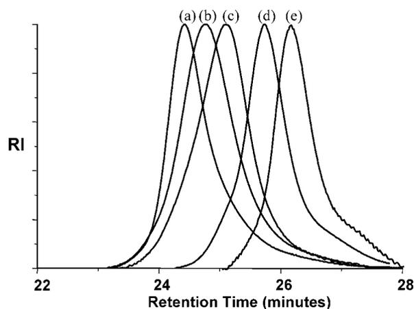
**Figure 3.** Overlay of GPC traces for (a) the starting linear polymer, **8**,  $M_w = 105\,000$ , PDI = 1.12; and nanoparticles, **9**, with (a) 0 mol % BCB incorporation, (b) 5 mol % BCB incorporation, (c) 10 mol % BCB incorporation, (d) 20 mol % BCB incorporation, and (e) 25 mol % BCB incorporation.
