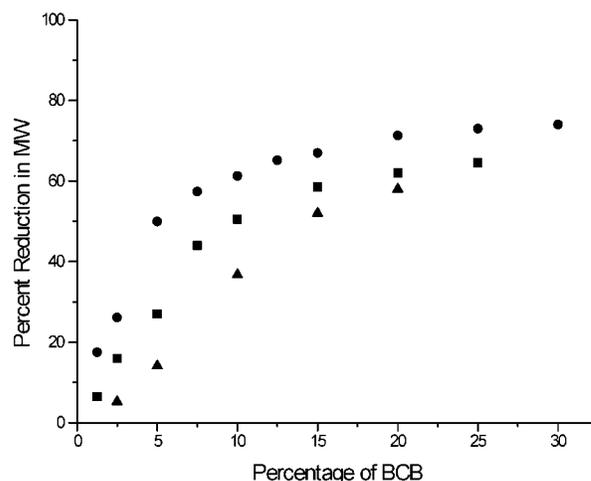
**Figure 4.** Variation in the percent reduction in molecular weight<sup>21</sup> for the nanoparticles, **9**, with the mol % of BCB units in the starting linear polymer, **8**, for 44 K (●), 110 K (■), and 230 K (▲) series.**Table 2.** Comparison of Molecular Weight (Linear Standard Equivalent) and PDI for the Starting Functionalized Linear Polymers, **10**, and the Final Nanoparticles, **11**
