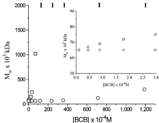
**Figure 1.** Variation in molecular weight of final macromolecule,  $M_w$ , with total concentration of BCB groups in solution; (□) ultra-high dilution strategy; (○) continuous addition strategy; (I) represents that an insoluble gel was produced (starting linear polymer;  $M_w = 95\,000$ ; PDI = 1.11).
