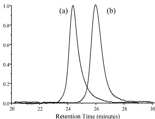
**Figure 5.** GPC traces for (a) the starting poly(ethylene glycol)-*b*-poly(styrene-*co*-benzocyclobutene), **15**, ( $M_w = 95\,000$ , PDI = 1.11) and (b) the final hybrid nanoparticle-linear block copolymer, **16**, ( $M_w = 52\,000$ , PDI = 1.09).
