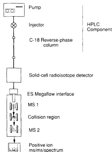
Figure 1. Schematic diagram of the HPLC/ES-MS/MS system.
