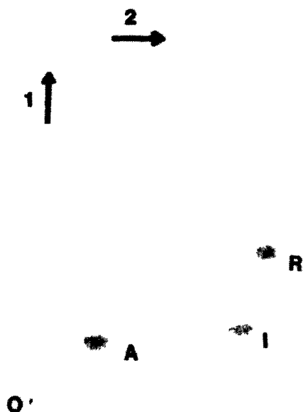
Fig. 2. Two-dimensional t.l.c. of Rib 5-P (R), D- g -D- alt -oct 1,8-P 2 (A), and D- g -D- ido -oct 1,8-P 2 (I), using the GW3 solvent 17 and then the GW3–2% PBA solvent. The chromatogram was developed twice in each direction, using the ascending mode. Sugar phosphates were visualised with the molybdate reagent 30 . The chromatogram was loaded with 0.05 \mu mol of R and 0.015 \mu mol of A and I. O' marks the origin.
