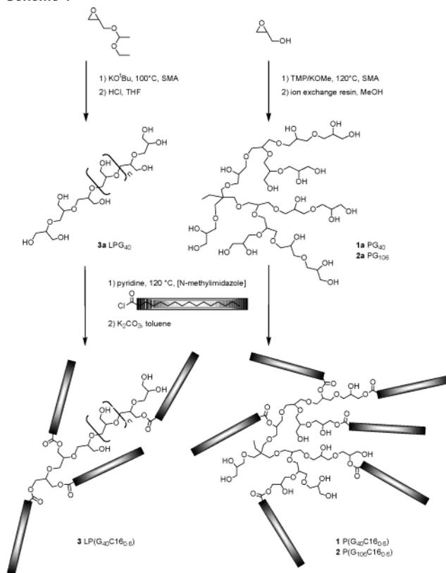
For the preparation of the linear analogue of the hyperbranched polyglycerols, a modification of a reported synthetic protocol<sup>11</sup> was applied, based on the slow addition of ethoxy ethyl glycidyl ether to KOtBu. After cleavage of the acetal groups, linear polyglycerol **3a** of narrow polydispersity ( $M_w/M_n = 1.3$ ) with a molecular weight of 3000 g/mol (VPO) was obtained.
