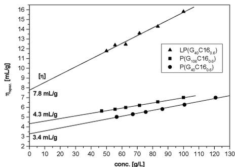
**Figure 2.** Specific viscosity vs concentration of **1–3** in toluene.
