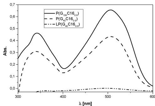
**Figure 1.** UV-vis spectra of **1**, **2**, and **3** (linear) after transfer of Congo Red dye into chloroform solution ( $[\text{Congo Red}]/[\text{polymer}] = 2$ ).
